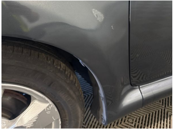
4: Wing nsf Poor Previous Repair Poor Paint
