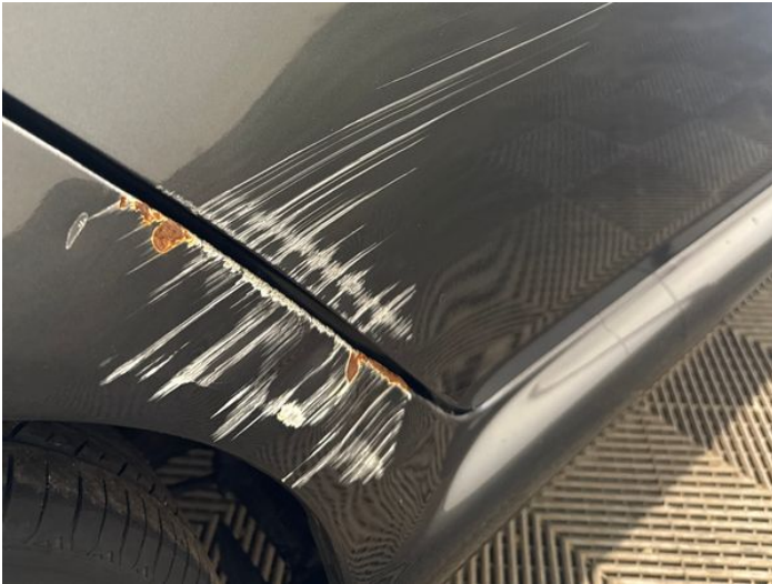
15: Door osr Dented With Paint Damage
