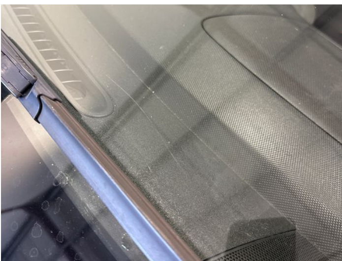
19: Screen Front Cracked Replace
