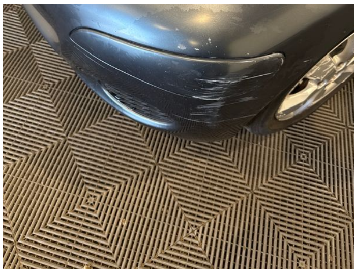
2: Bumper Front Poor Previous Repair Paint Flake
