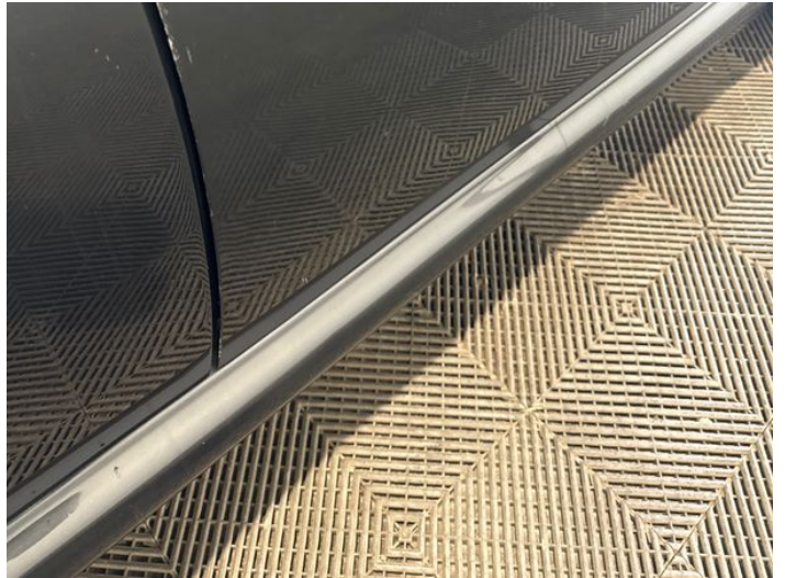
16: Door osf Scratched Over 25mm Thru Paint
