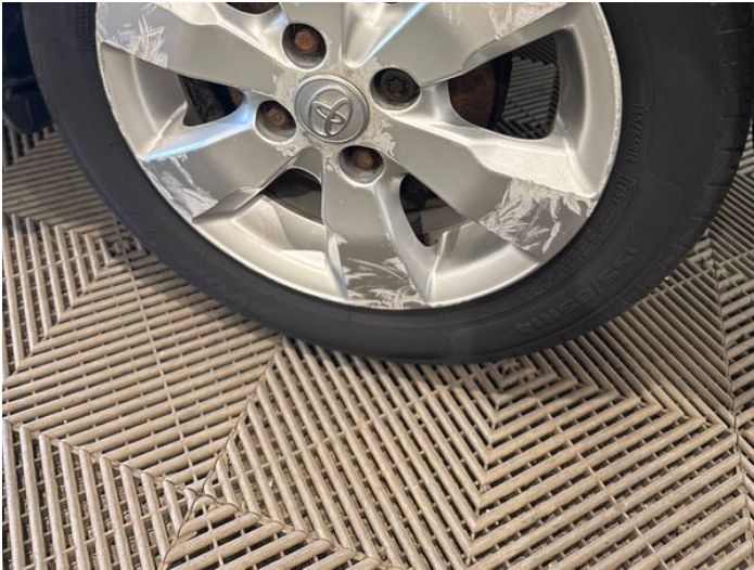
9: Wheel nsr Scratched Over 50mm
