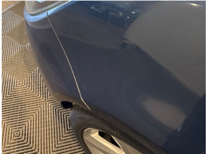
4: Wing nsf Scratched UpTo 25mm Thru Paint
