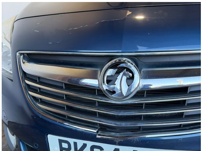
20: Bumper Front Grill Broken Replace
