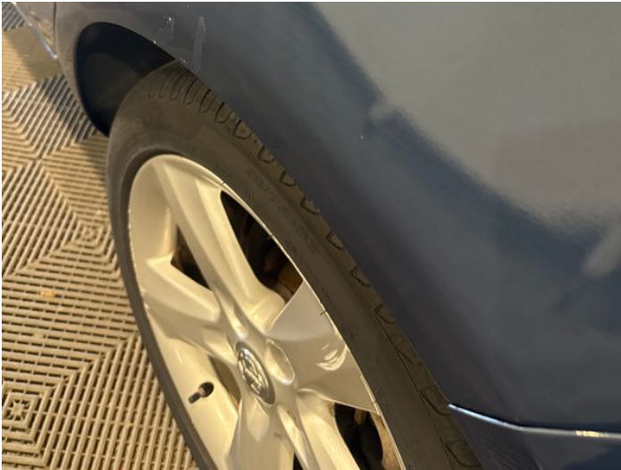
9: Qtr Panel nsr Poor Previous Repair Paint Flake
