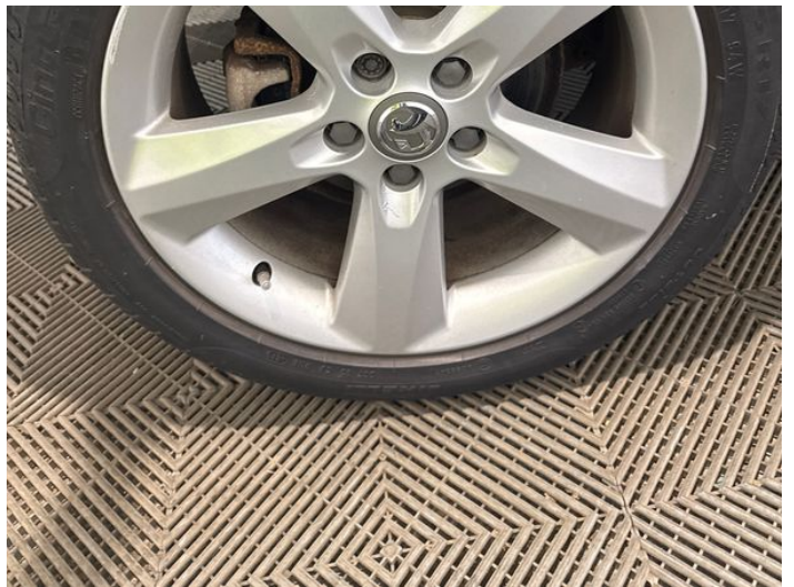
12: Wheel osr Scratched Over 50mm
