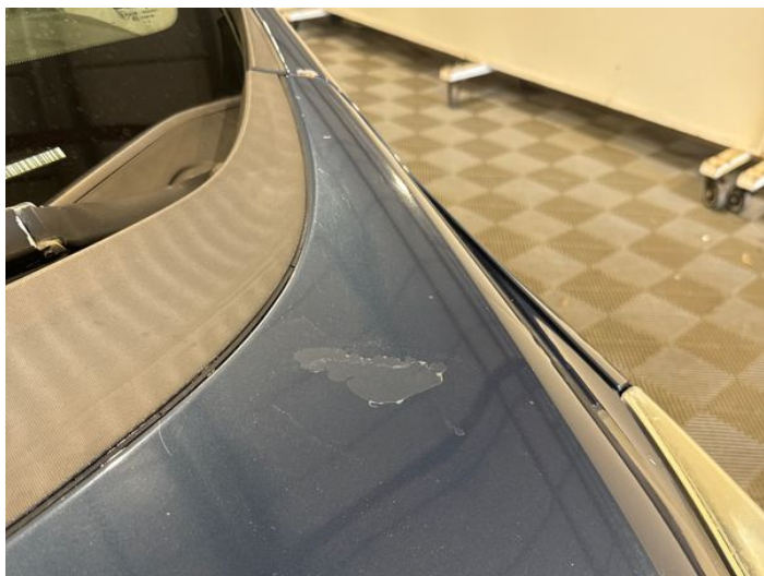
1: Bonnet Poor Previous Repair Paint Flake
