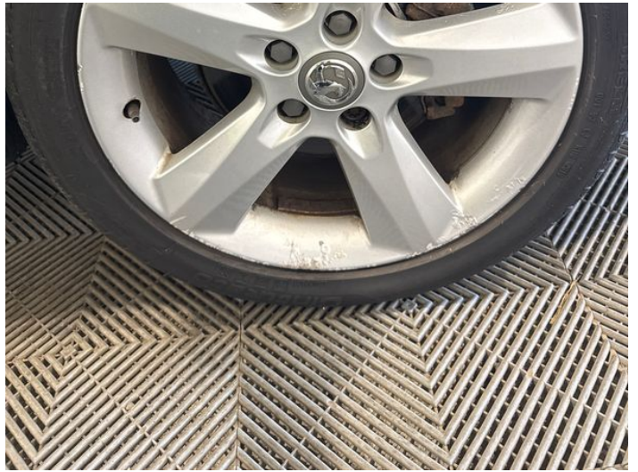
18: Wheel osf Scratched Over 50mm
