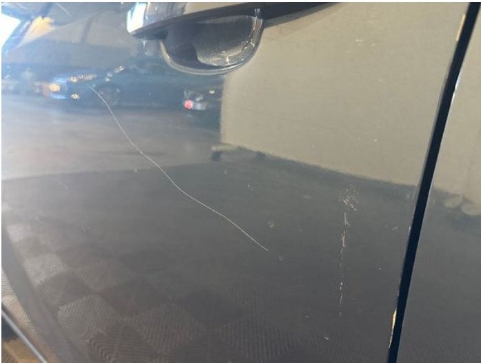
5: Door nsf Scratched Over 25mm Thru Paint
