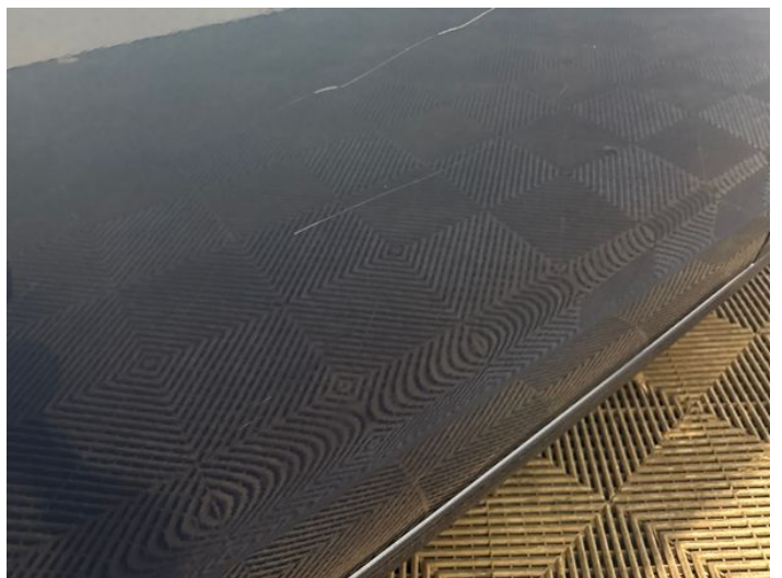
14: Door osr Scratched Over 25mm Thru Paint
