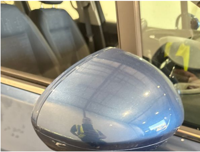
17: Door Mirror Assy osf Scratched (Painted) UpTo 25mm Thru Paint
