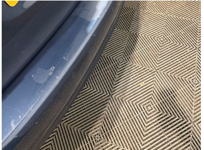
10: Bumper Rear Poor Previous Repair Paint Flake
