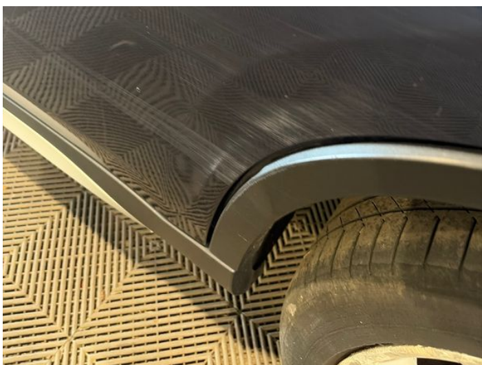
7: Door nsr Scratched Over 25mm Thru Paint
