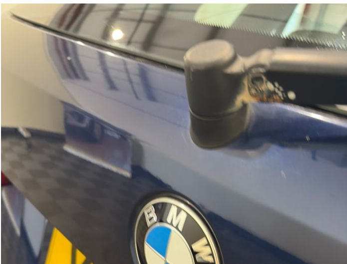
13: Tailgate Scratched UpTo 25mm Thru Paint
