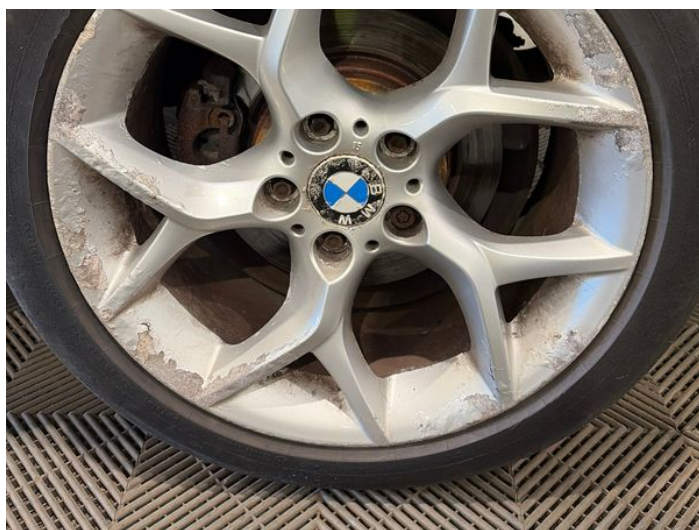
8: Wheel nsr Scratched Over 50mm
