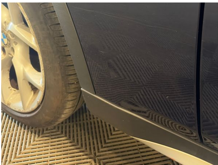
5: Wing nsf Scratched UpTo 25mm Thru Paint
