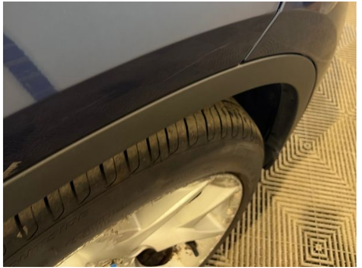
18: Wing osf Scratched Over 25mm Thru Paint
