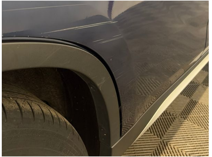
16: Door osr Scratched Over 25mm Thru Paint
