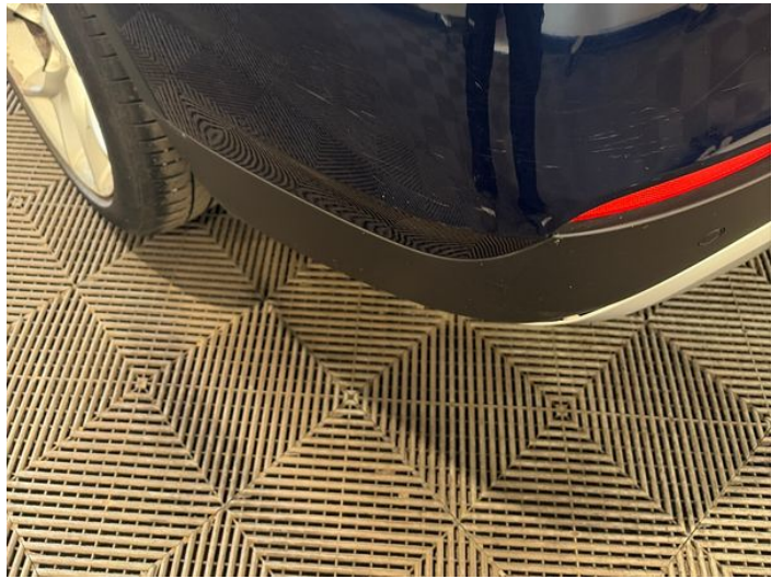
12: Bumper Rear Scratched Over 100mm Thru Paint
