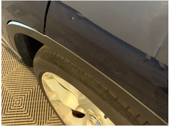
10: Qtr Panel nsr Dented Between 10mm + 30mm
