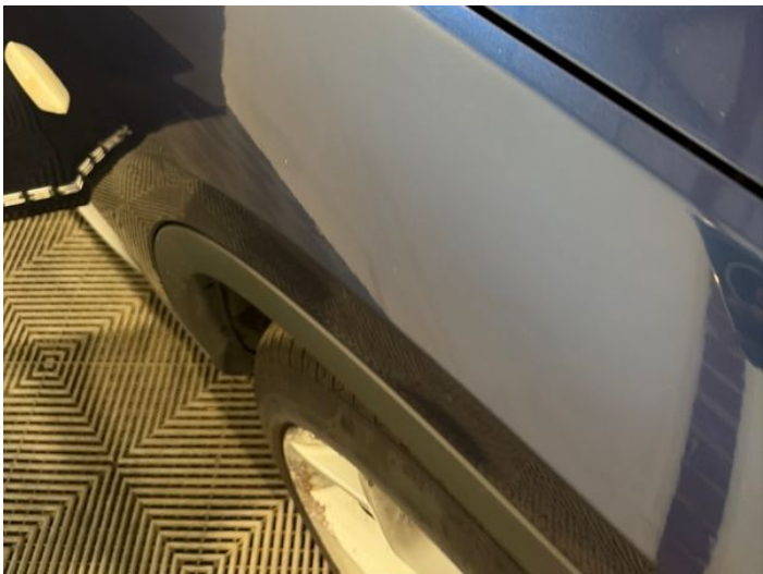
22: Wing of Dented Between 10mm + 30mm
