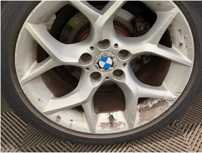
15: Wheel osr Scratched Over 50mm
