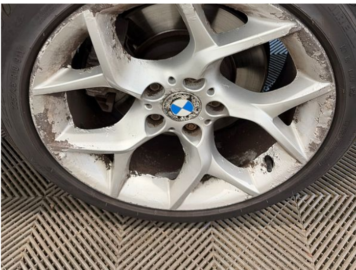
19: Wheel osf Corroded Light
