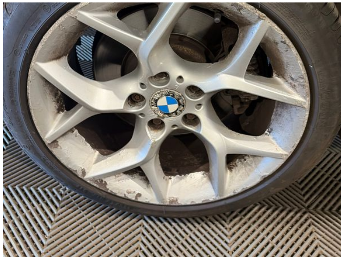
4: Wheel nsf Scratched Over 50mm
