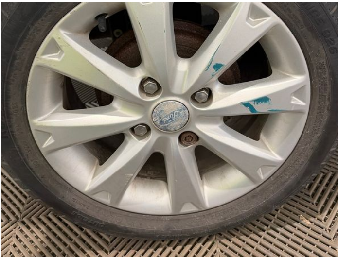
17: Wheel osr Scratched Over 50mm
