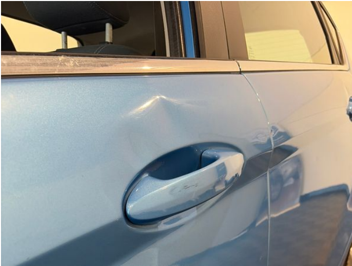
9: Door nsf Dented With Paint Damage
