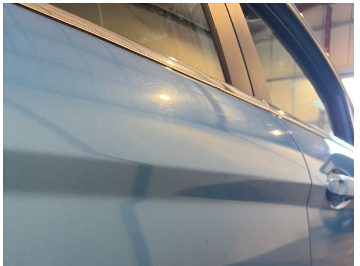
18: Door osr Dented Over 30mm
