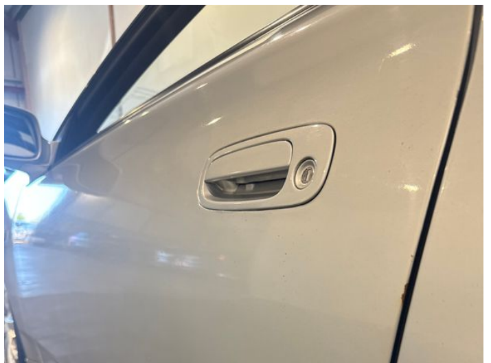
8: Door nsf Poor Previous Repair Rippled UpTo 30%
