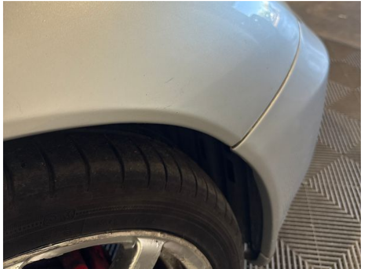
16: Wing osf Poor Previous Repair Poor Paint
