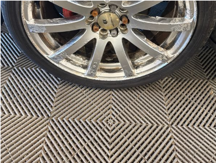
3: Wheel nsf Corroded Light
