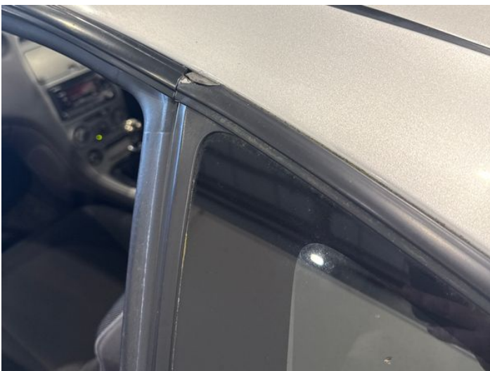
7: Aperture Seal nsr Broken Replace
