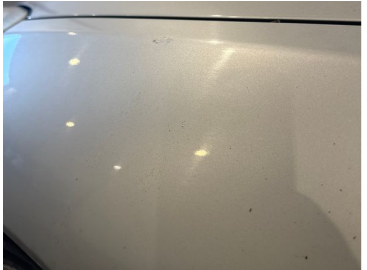
4: Wing nsf Scratched UpTo 25mm Thru Paint
