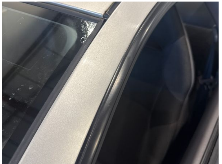
6: A Post nsf Scratched UpTo 25mm Thru Paint
