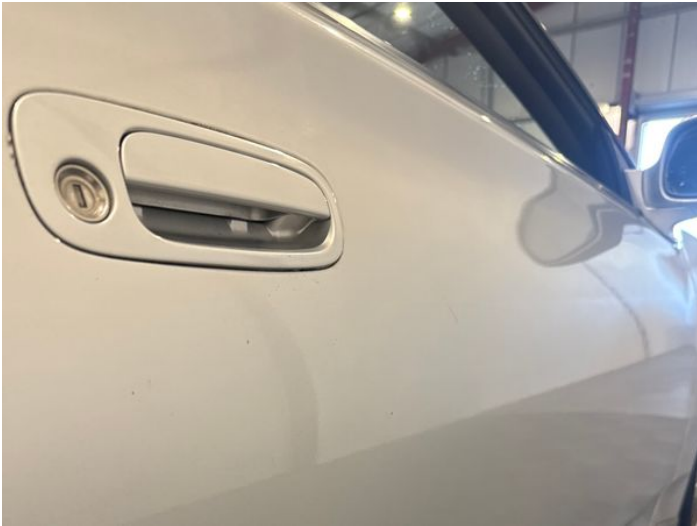
15: Door osf Poor Previous Repair Rippled UpTo 30%
