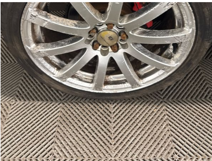
13: Wheel osr Corroded Light
