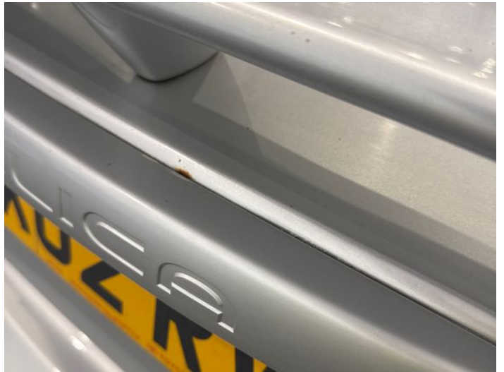
12: Tailgate Rusted Over 5mm
