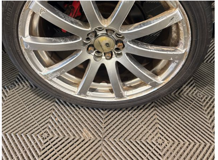
10: Wheel nsr Corroded Light
