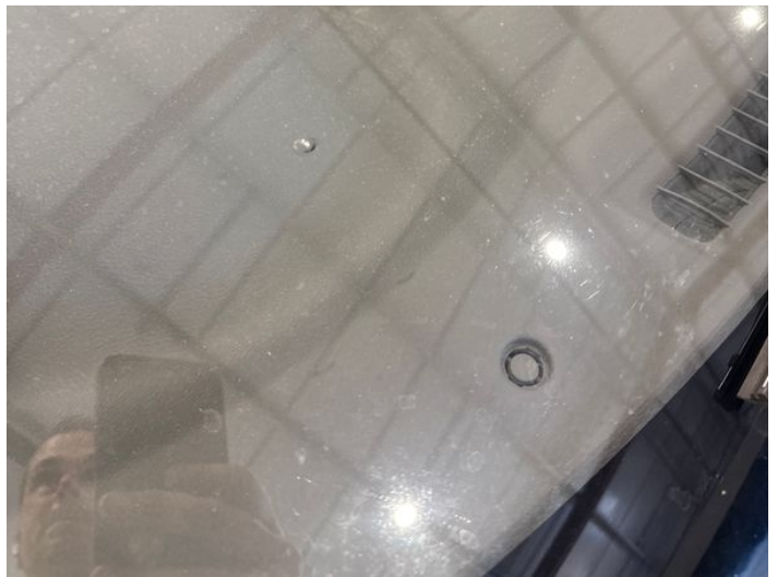
18: Screen Front Chipped Over 10mm
