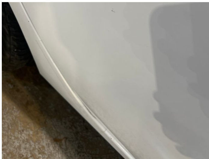
2: Door osr Chipped 1 To 5
