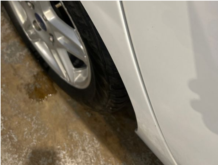
3: Qtr Panel osr Dented Over 30mm
