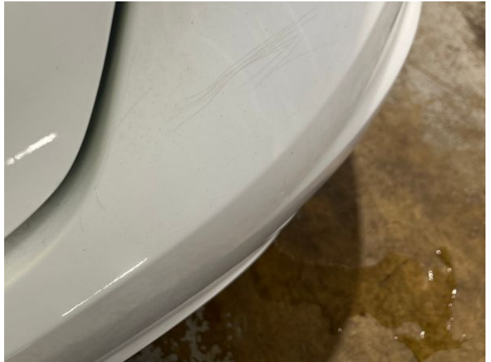
4: Bumper Rear Poor Previous Repair Paint Flake
