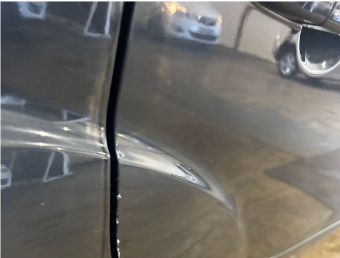
5: Door osr Chipped Edge Chip
