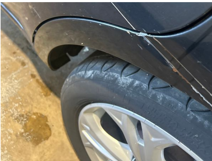
13: Door nsr Scratched Over 25mm Thru Paint
