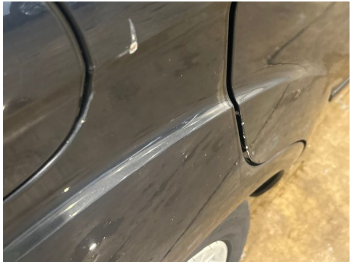
6: Qtr Panel osr Scratched UpTo 25mm Thru Paint
