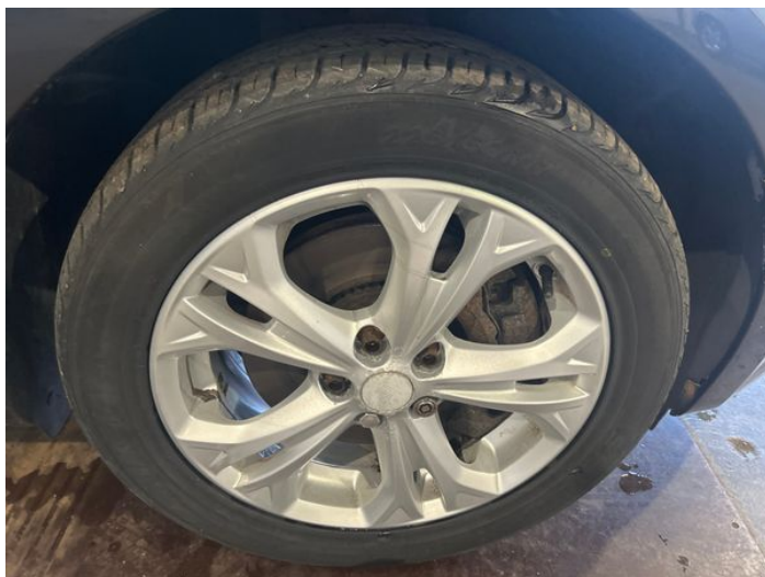
1: Wheel osf Corroded Light
