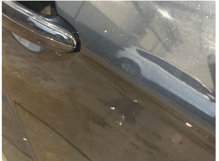
4: Door osr Chipped 1 To 5
