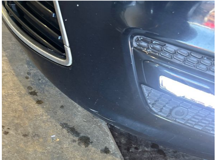
16: Bumper Front Scratched Over 100mm Thru Paint
