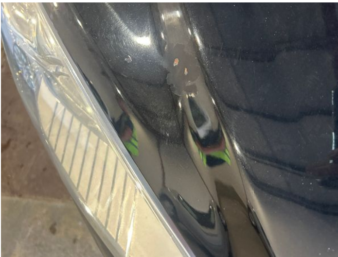
17: Bonnet Poor Previous Repair Paint Flake
