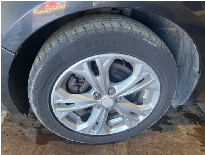
15: Wheel nsf Scratched Over 50mm
