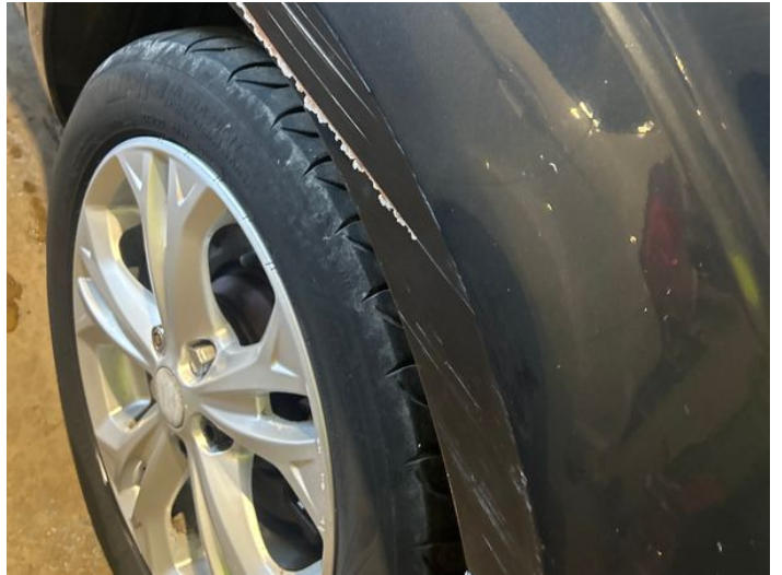
10: Qtr Panel nsr Dented With Paint Damage
