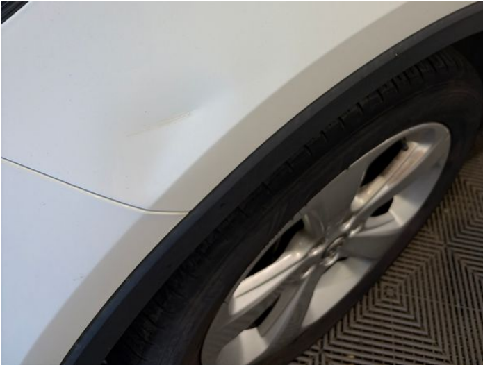
3: Wing nsf Dented With Paint Damage
