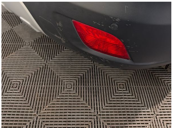
8: Bumper Rear Moulding Scuffed (Unpainted) UpTo 100mm
