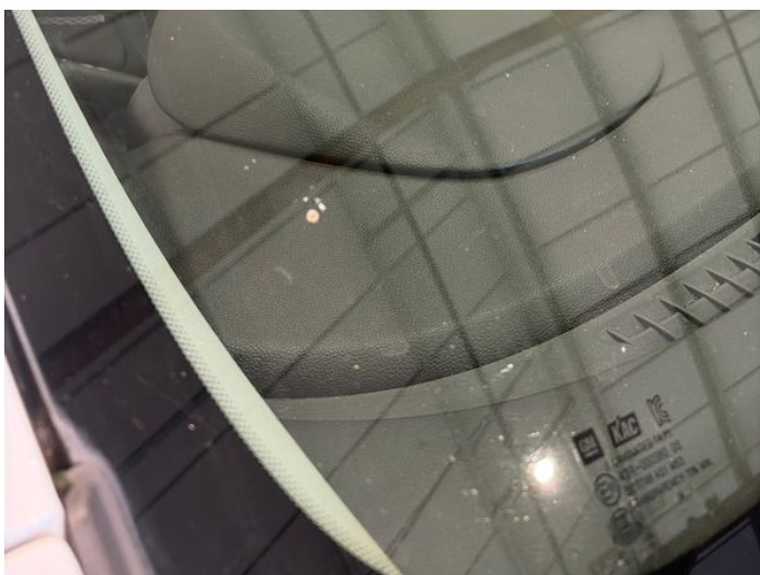
13: Screen Front Chipped UpTo 10mm
