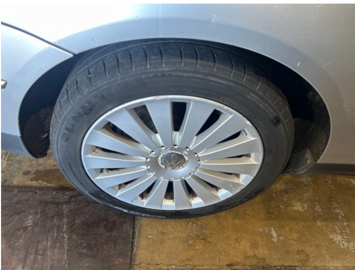
7: Wheel osr Scratched Over 50mm
