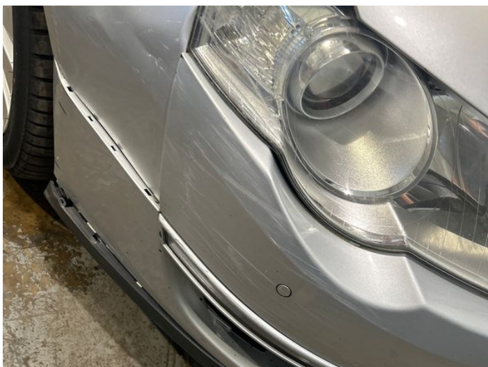
17: Bumper Front Scratched 25 to 100mm Thru Paint
