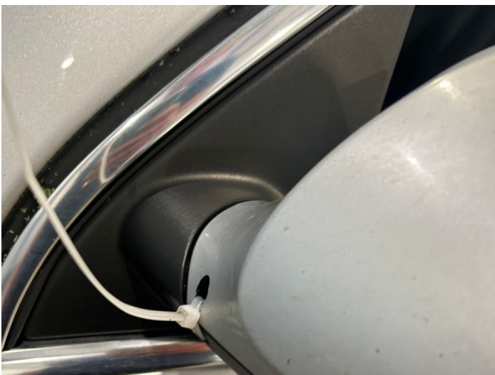
13: Door Mirror Assy nsf Broken Replace
