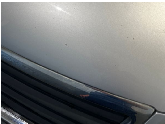
16: Bonnet Chipped Multiple Chips
