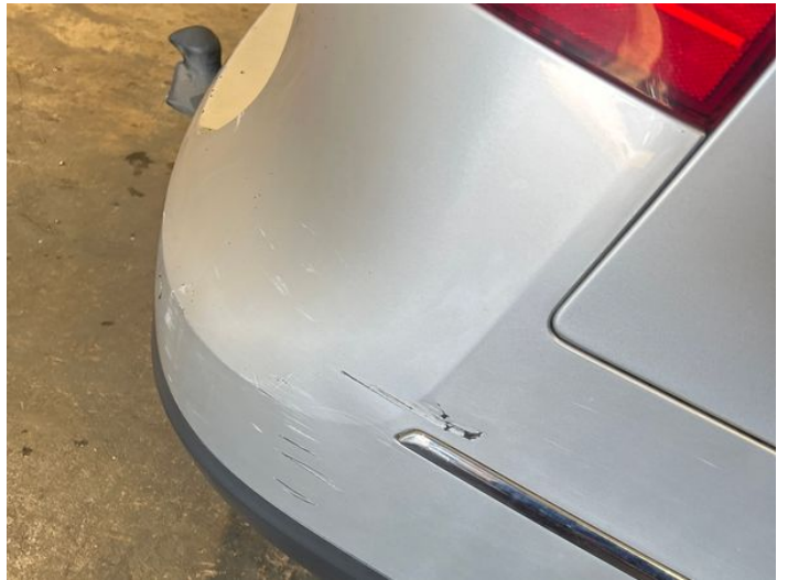
6: Bumper Rear Scratched Over 100mm Thru Paint
