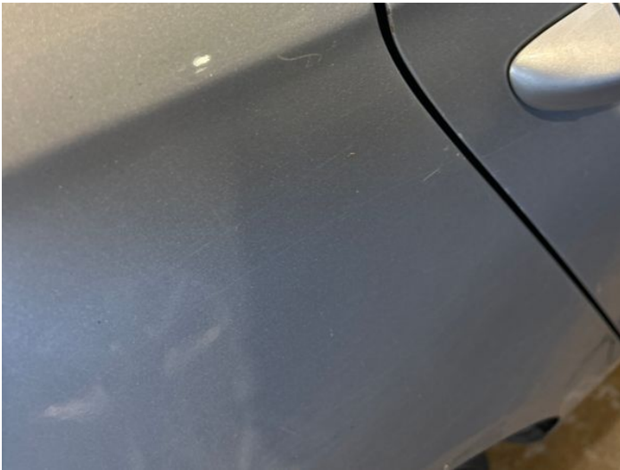
5: Qtr Panel osr Scratched UpTo 25mm Thru Paint
