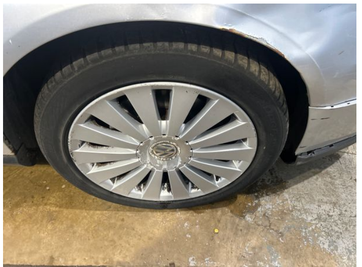
8: Wheel osf Scratched Over 50mm
