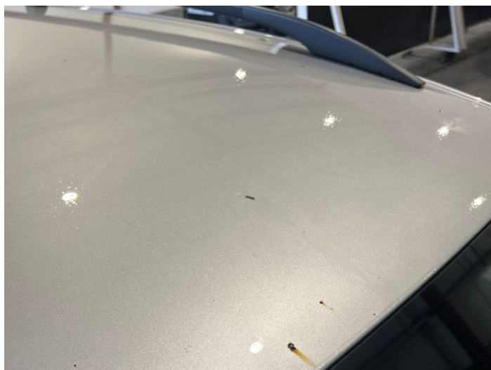
18: Roof Chipped 1 To 5
