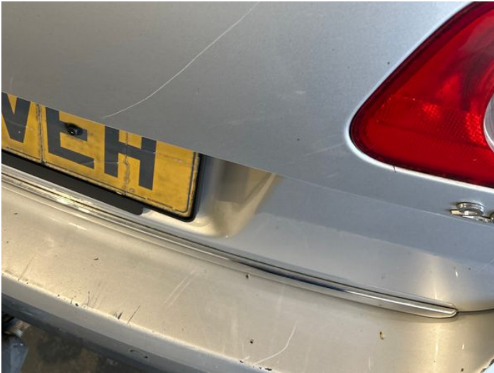
9: Tailgate Scratched Over 25mm Thru Paint
