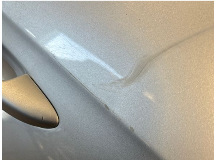
4: Door osr Scratched Over 25mm Thru Paint
