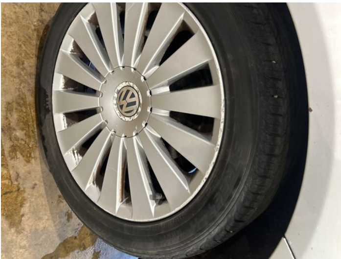
11: Wheel nsr Scratched Over 50mm
