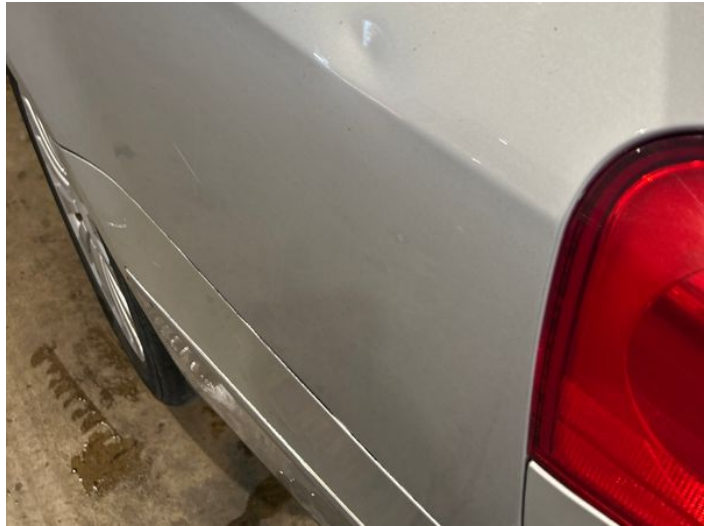
10: Qtr Panel nsr Dented Over 30mm
