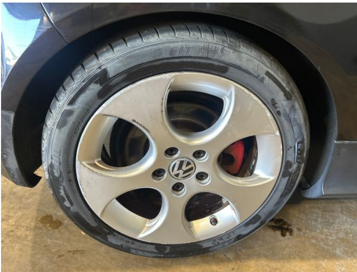
5: Wheel osr Scratched Over 50mm
