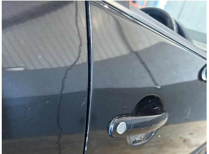
4: Door osf Chipped Edge Chip
