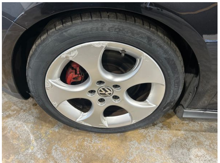
14: Wheel nsf Scratched Over 50mm
