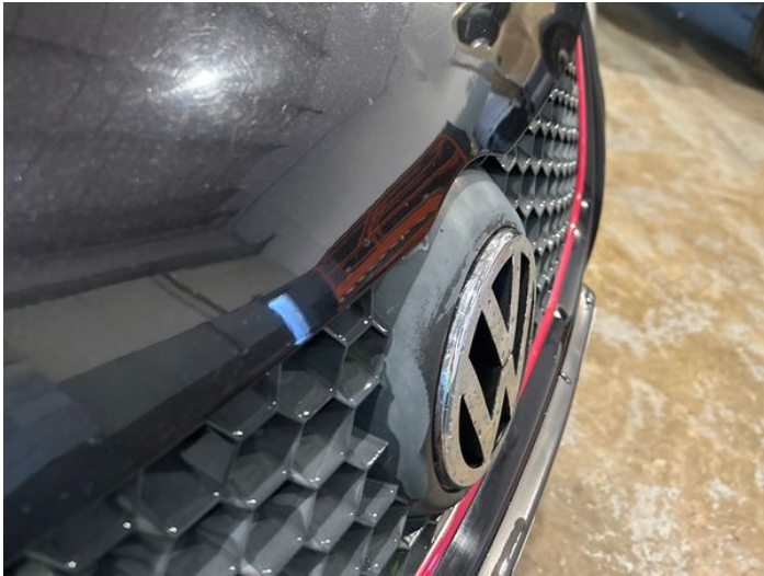
16: Bonnet Dented Over 30mm
