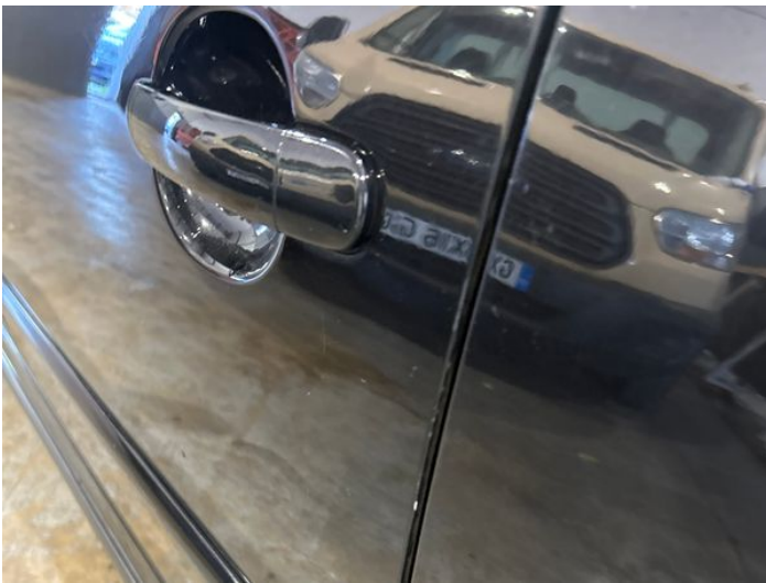
11: Door nsf Chipped Edge Chip
