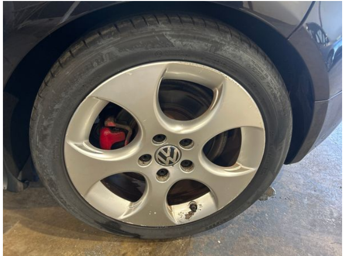
10: Wheel nsr Corroded Light
