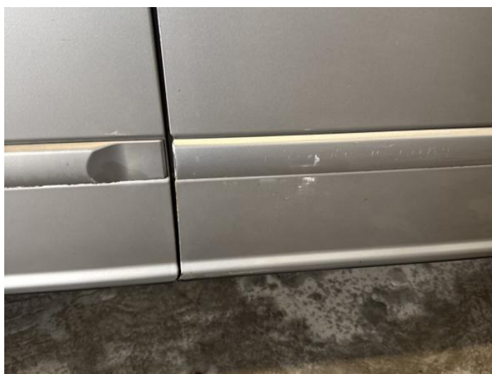
6: Door osf Rusted UpTo 5mm
