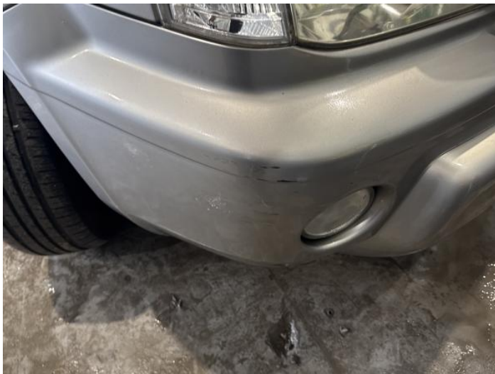
9: Bumper Front Scratched Over 100mm Thru Paint
