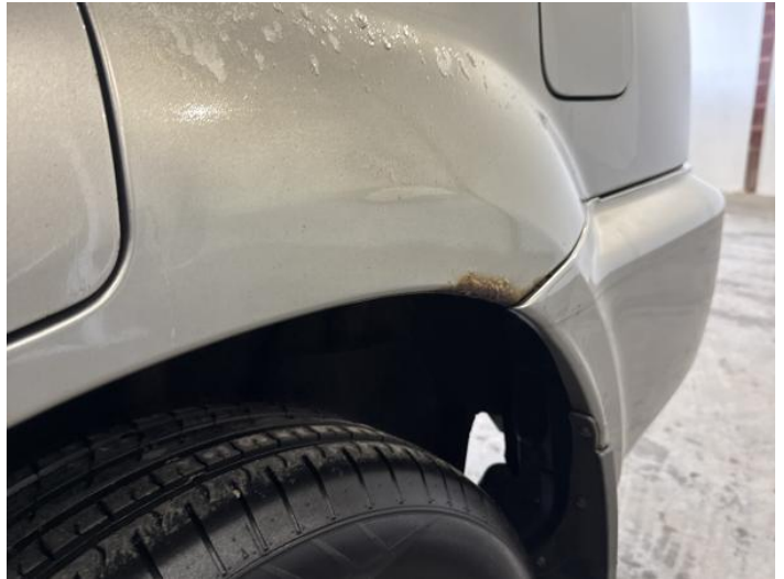
16: Qtr Panel nsr Rusted Over 5mm
