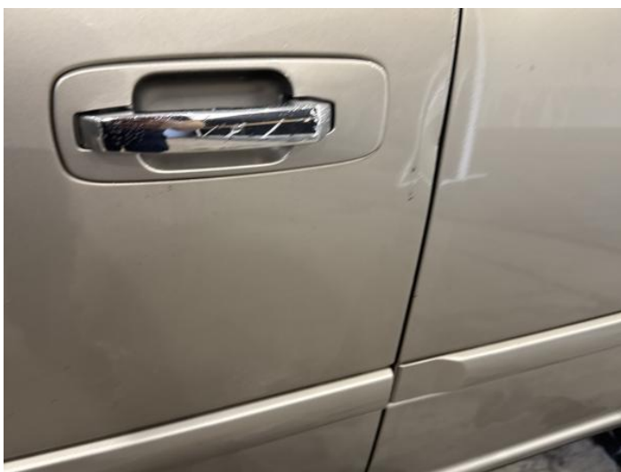
13: Door nsf Dented With Paint Damage
