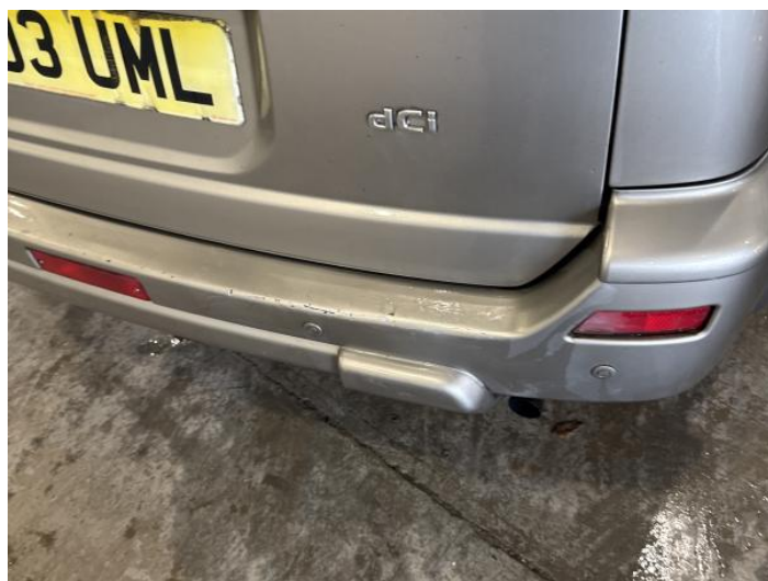
1: Bumper Rear Scratched Over 100mm Thru Paint
