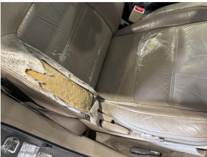
19: Seat Back Cover osf Torn Over 3mm
