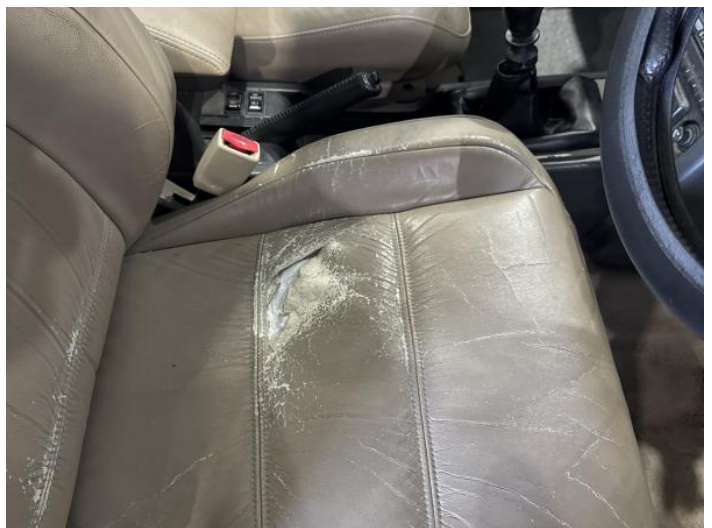
20: Seat Base Cover osf Torn Over 3mm
