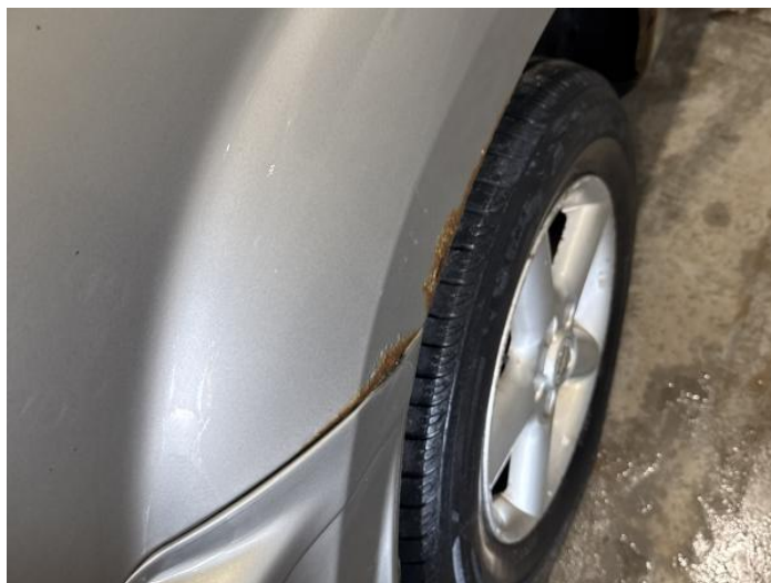
4: Qtr Panel osr Rusted Over 5mm
