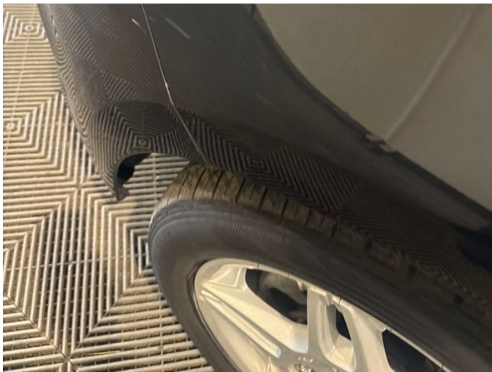
3: Wing nsf Scratched Over 25mm Thru Paint
