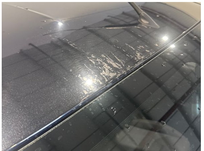
20: Roof Scratched Over 25mm Thru Paint
