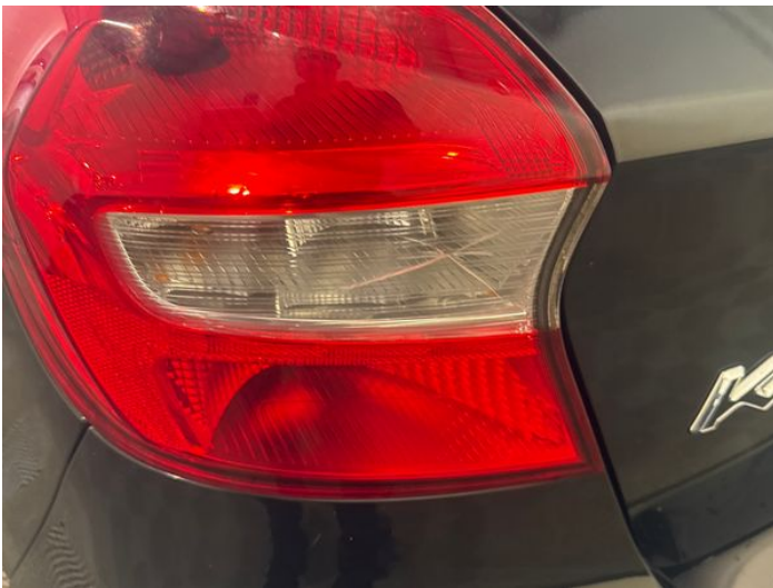
11: Lamp nsr Broken Replace
