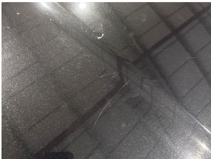
1: Bonnet Scratched Over 25mm Thru Paint
