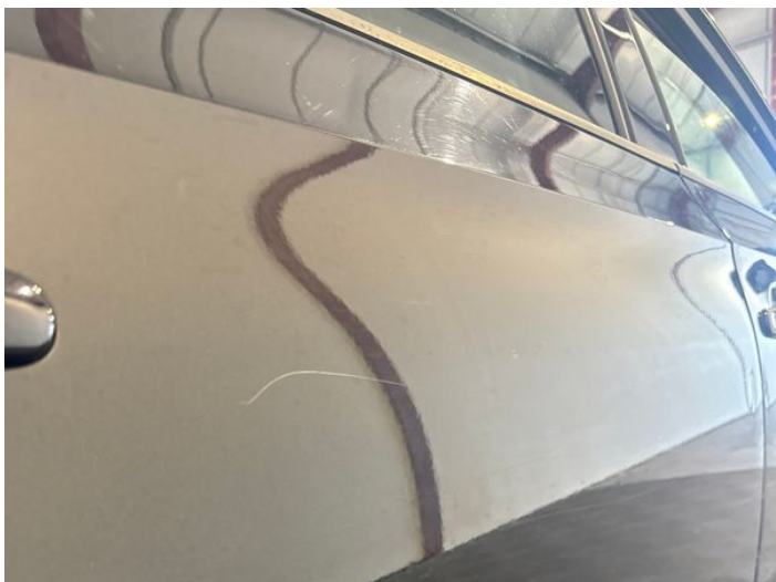
15: Door osr Scratched Over 25mm Thru Paint
