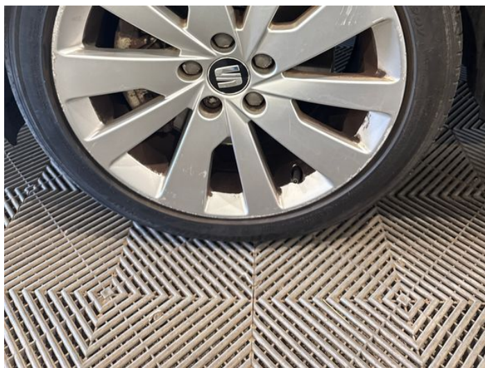
6: Wheel nsf Scratched Over 50mm
