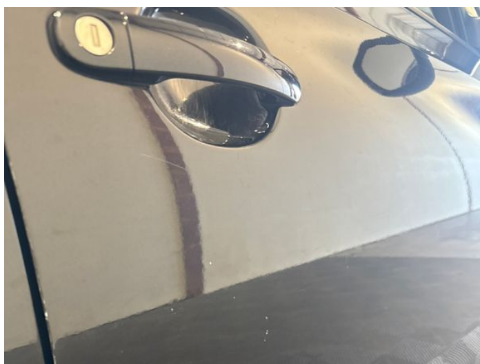
18: Door osf Scratched Over 25mm Thru Paint
