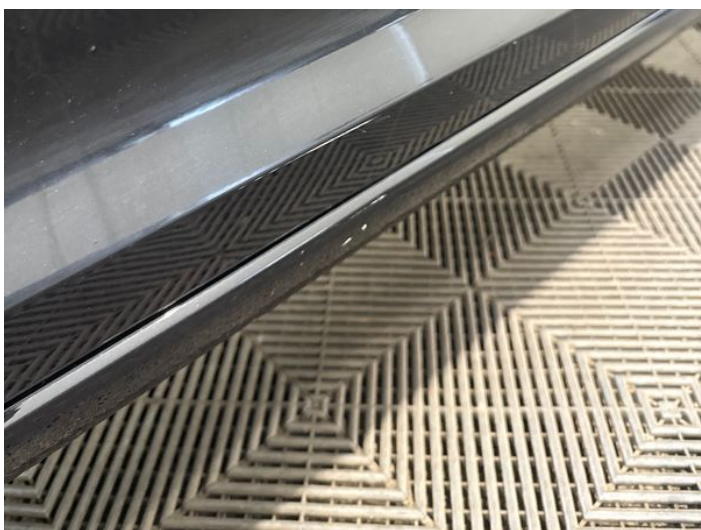
7: Door nsf Scratched Over 25mm Thru Paint
