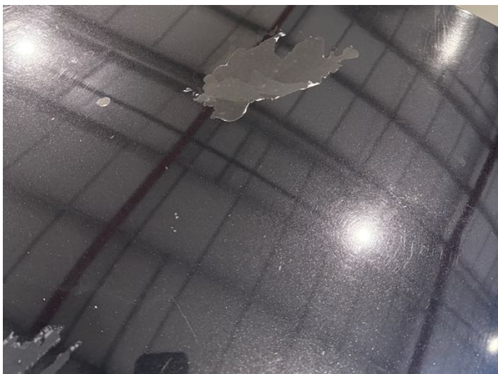
3: Bonnet Poor Previous Repair Paint Flake
