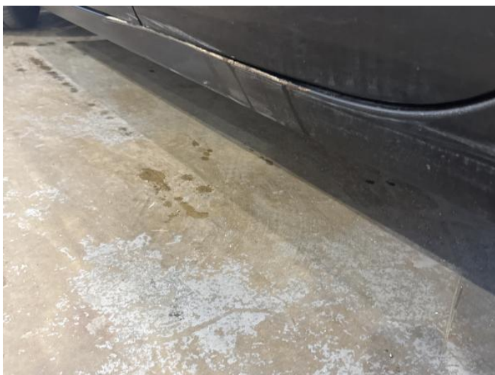
11: Sill ns Dented With Paint Damage
