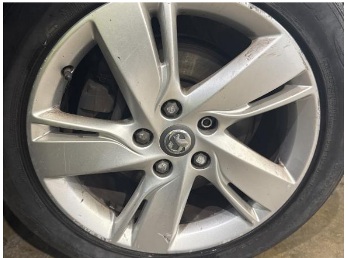
6: Wheel nsf Scratched Over 50mm
