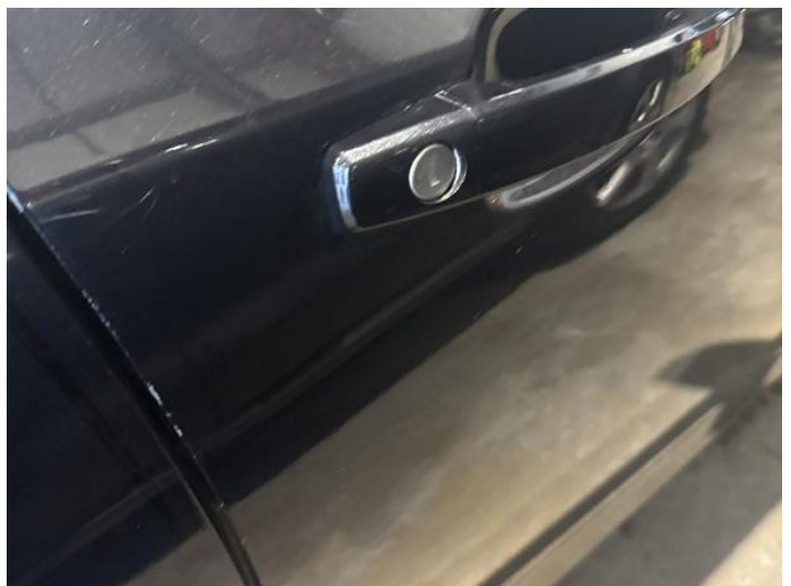
20: Door osf Scratched Over 25mm Thru Paint
