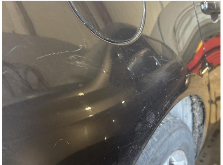
16: Qtr Panel osr Dented With Paint Damage
