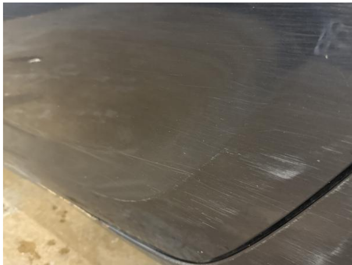
10: Door nsr Scratched Over 25mm Thru Paint
