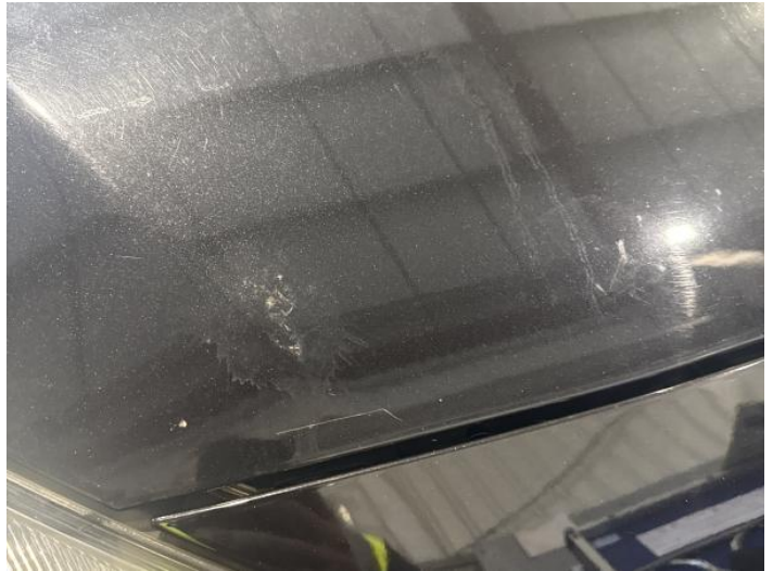
4: Bonnet Scratched Over 25mm Thru Paint
