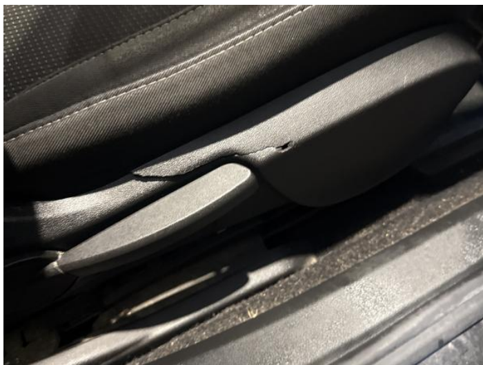
1: Fascia Trim Damaged Replace
