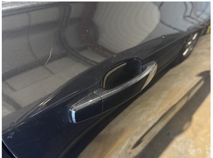
18: Door osr Scratched Over 25mm Thru Paint
