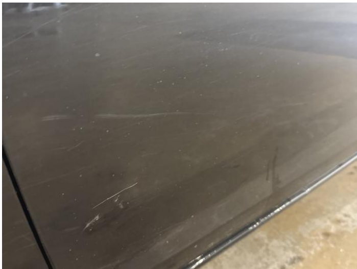
9: Door nsf Dented With Paint Damage
