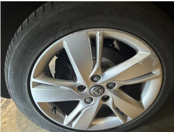
17: Wheel osr Scratched Over 50mm
