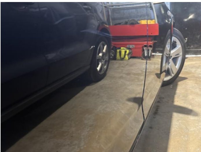
19: Door osr Dented Between 10mm + 30mm
