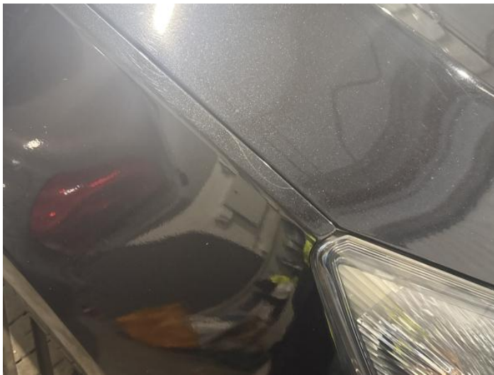
21: Wing osf Scratched Over 25mm Thru Paint
