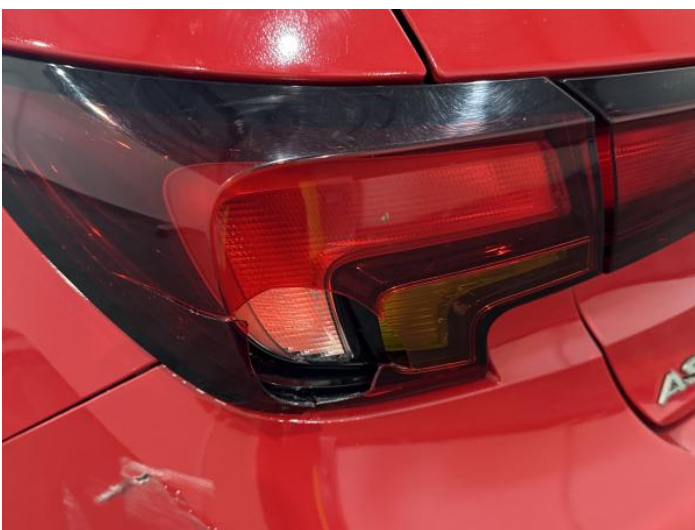
13: Lamp nsr Broken Replace
