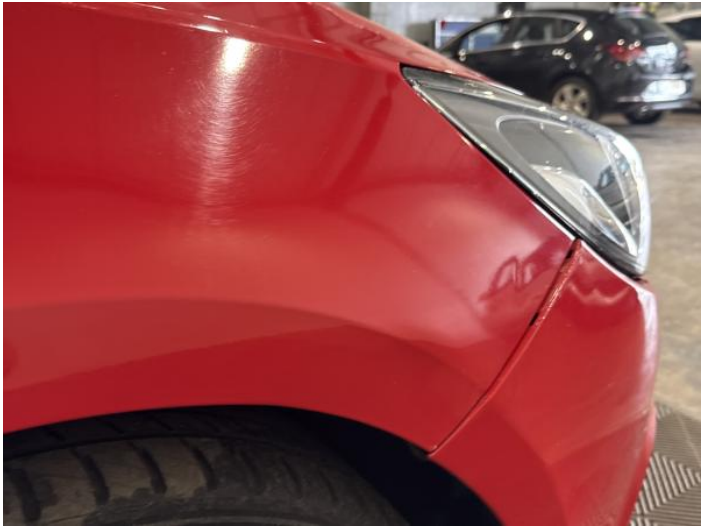
22: Wing osf Dented Over 30mm
