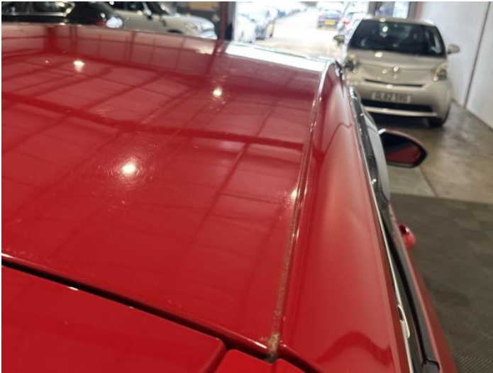
15: Roof Dented Over 30mm
