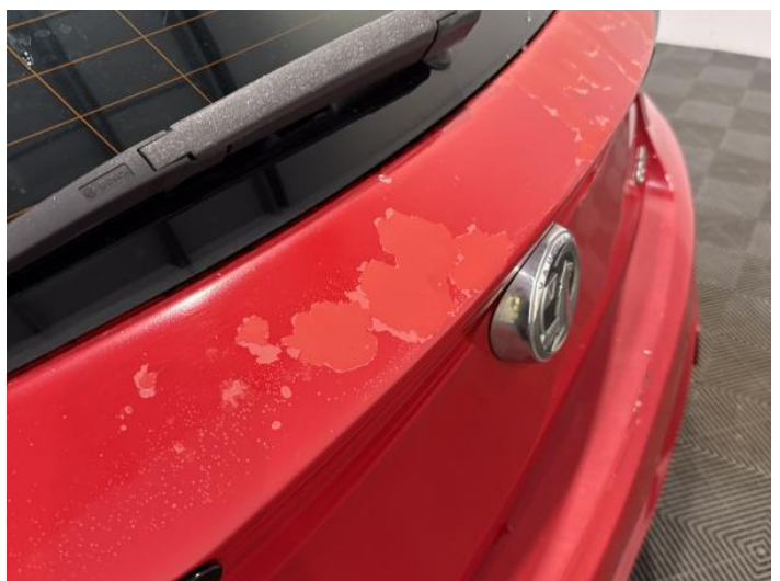
14: Tailgate Poor Previous Repair Paint Flake
