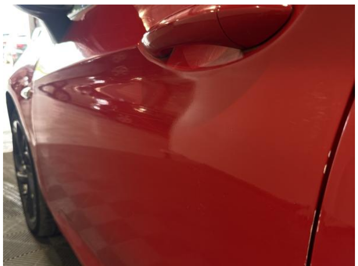
8: Door nsf Poor Previous Repair Rippled UpTo 30%
