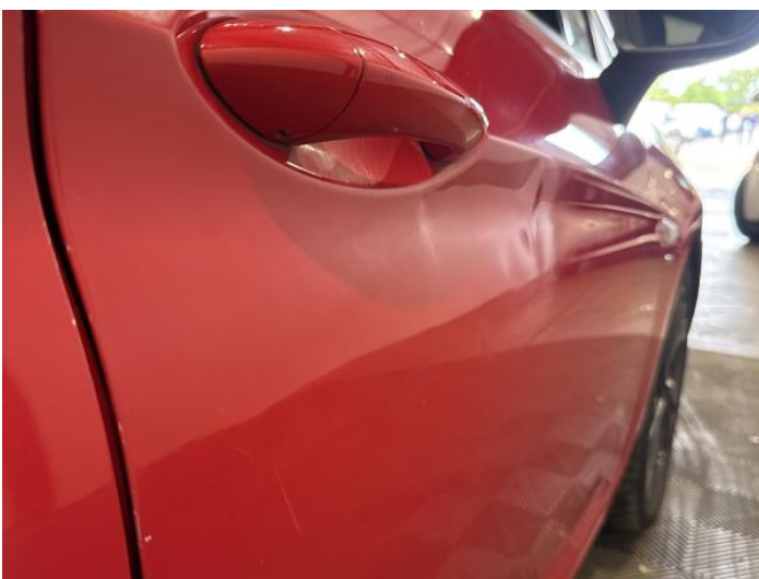
19: Door osf Poor Previous Repair Rippled UpTo 30%
