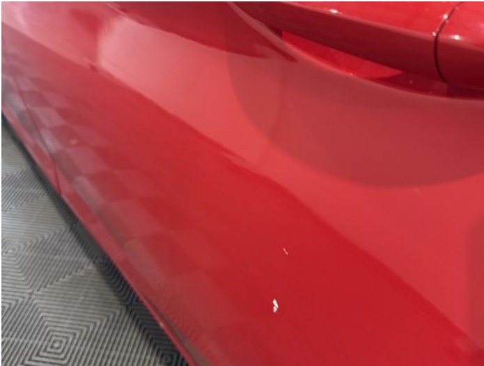
9: Door nsr Poor Previous Repair Rippled UpTo 30%
