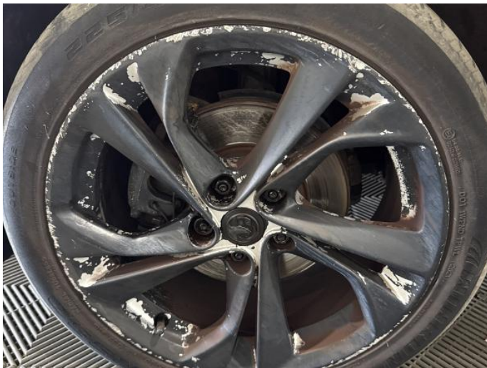
5: Wheel nsf Scratched Over 50mm
