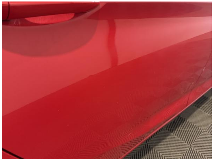
18: Door osr Dented Over 30mm
