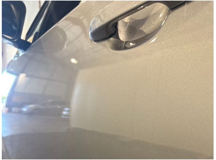
4: Door nsf Poor Previous Repair Rippled Up To 30%
