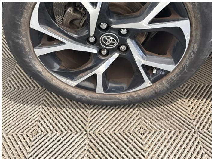
8: Wheel osr Scratched Over 50mm
