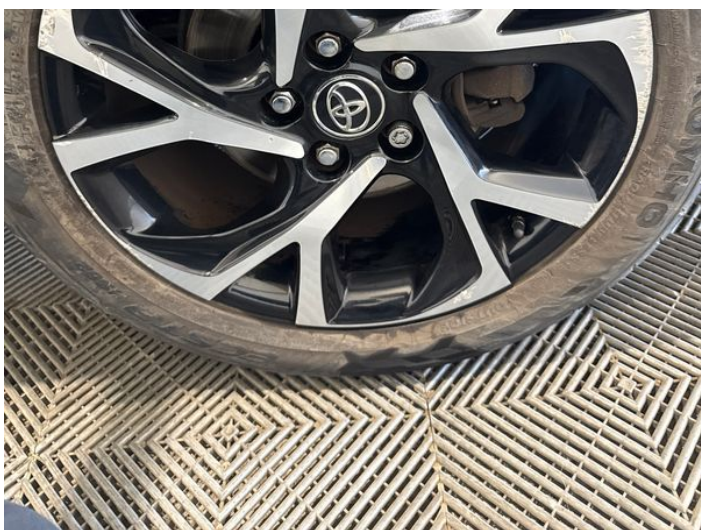
13: Wheel osf Scratched Over 50mm
