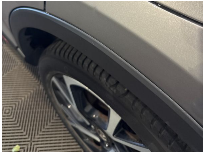
6: Qtr Panel nsr Dented Between 10mm + 30mm
