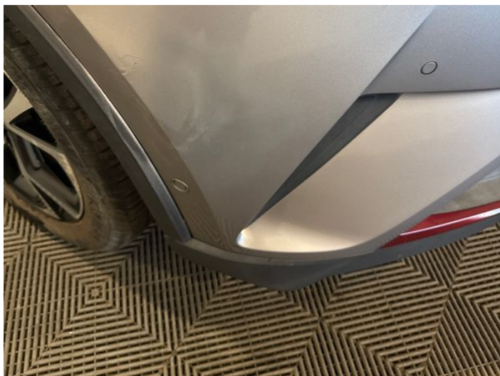
1: Bumper Front Poor Previous Repair Poor Paint
