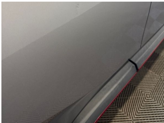
10: Door osr Scratched UpTo 25mm Thru Paint
