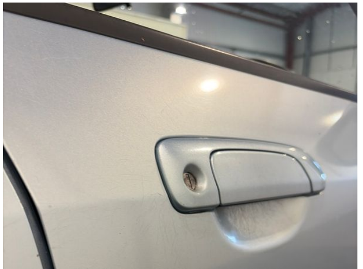
18: Door osf Scratched Over 25mm Thru Paint
