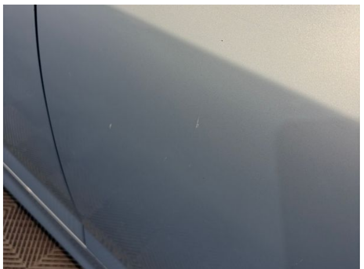
8: Door nsr Scratched UpTo 25mm Thru Paint
