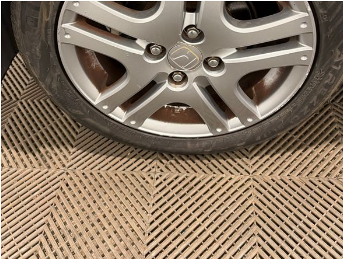
15: Wheel osr Scratched Over 50mm
