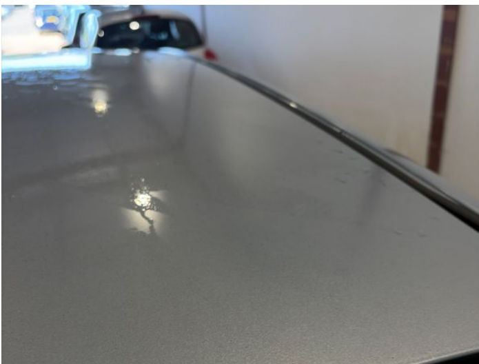
13: Roof Dented 2 Or Less UpTo 10mm
