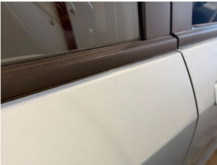
17: Door osr Dented With Paint Damage
