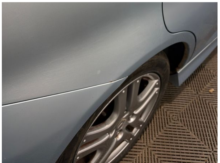
14: Qtr Panel osr Poor Previous Repair Rippled UpTo 30%
