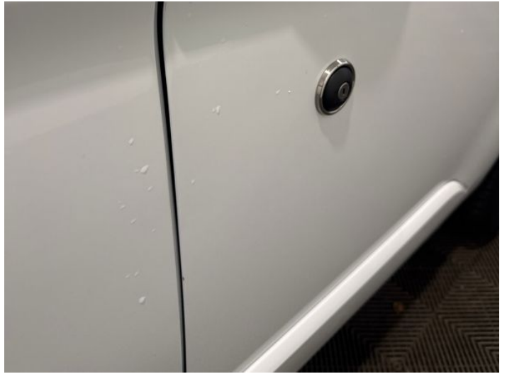
16: Door osf Chipped Edge Chip
