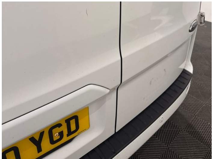
12: Tailgate Dented With Paint Damage
