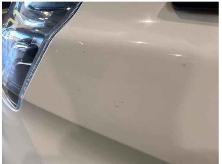
6: Wing nsf Scratched Over 25mm Thru Paint
