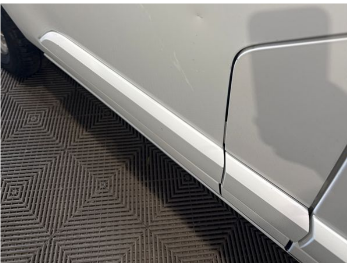
7: Door nsf Dented With Paint Damage
