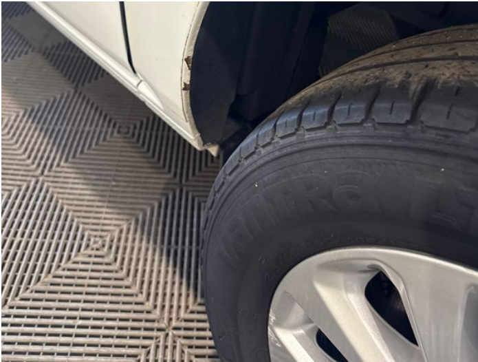
9: Qtr Panel nsr Rusted Over 5mm
