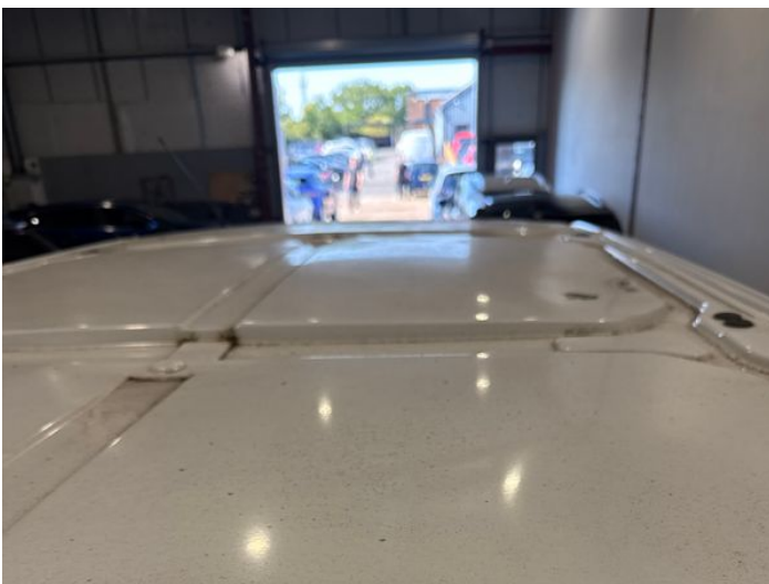
13: Roof Dented Over 30mm
