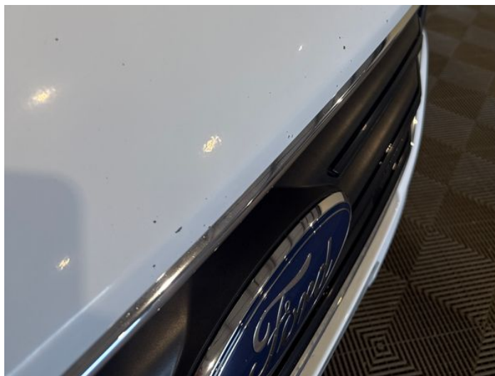
2: Bonnet Dented With Paint Damage
