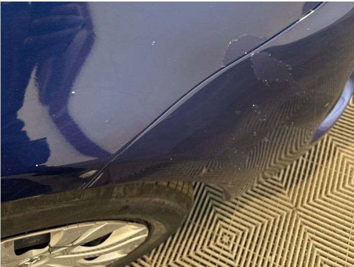
12: Wing osf Poor Previous Repair Paint Flake
