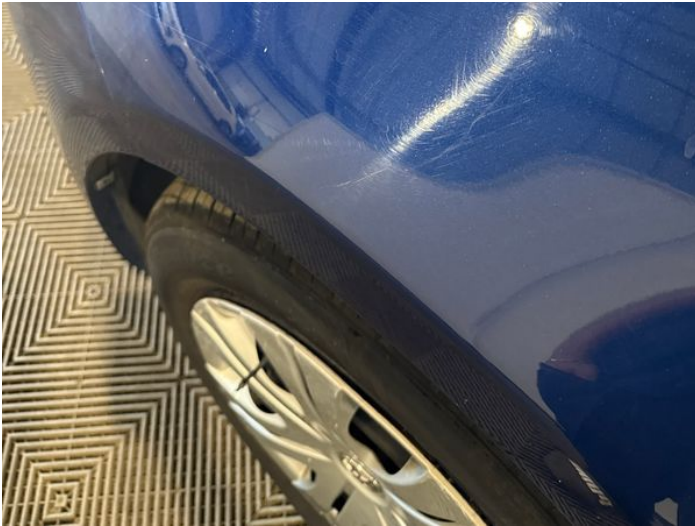
3: Wing nsf Scratched Over 25mm Thru Paint
