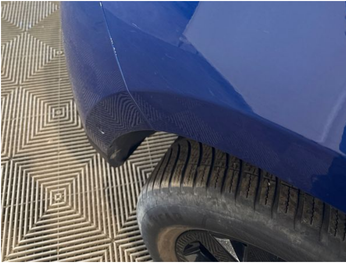
3: Wing nsf Scratched UpTo 25mm Thru Paint
