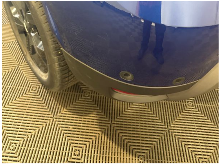
6: Bumper Rear Scratched 25 to 100mm Thru Paint
