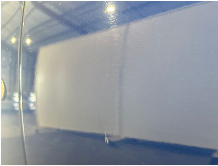
5: Door nsr Scratched UpTo 25mm Thru Paint
