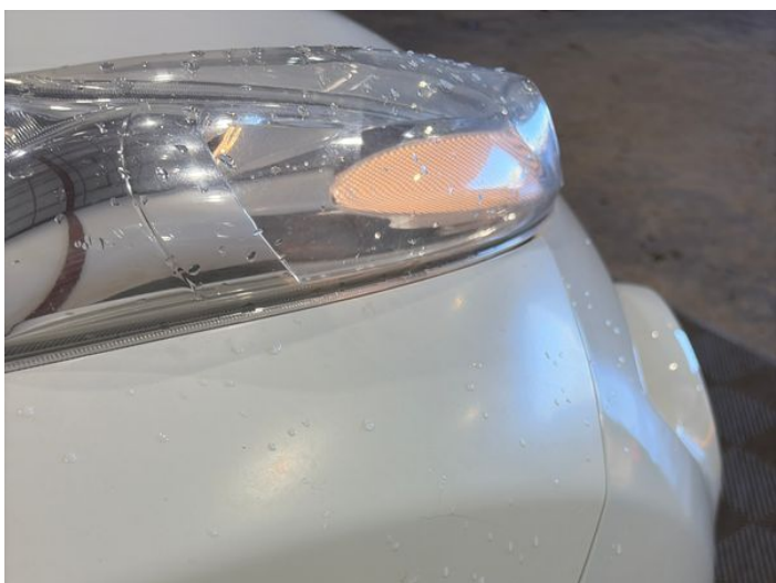
19: Wing osf Scratched Over 25mm Thru Paint
