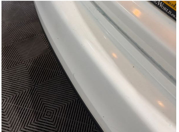
12: Bumper Rear Scratched 25 to 100mm Thru Paint
