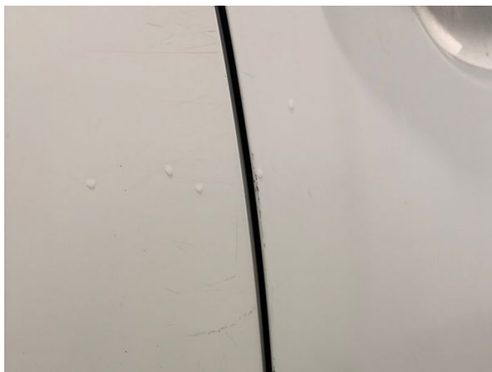
18: Door osr Scratched UpTo 25mm Thru Paint
