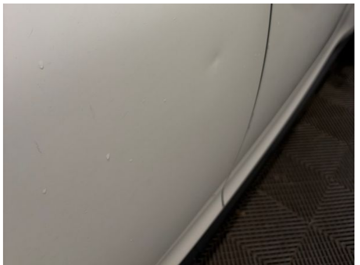
14: Door osr Dented Between 10mm + 30mm
