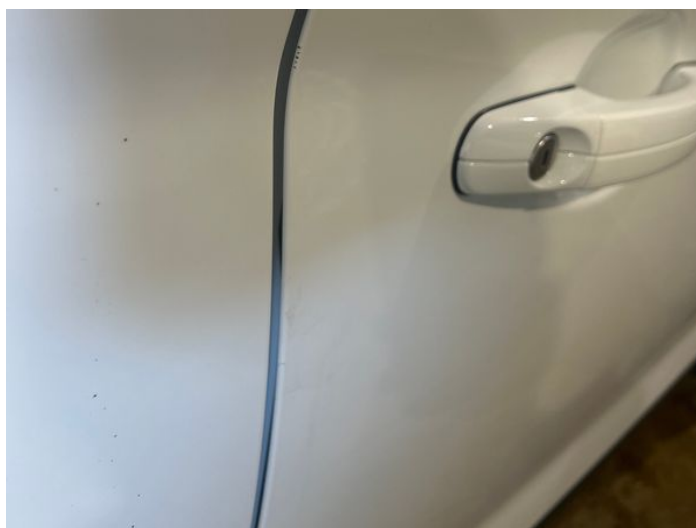
2: Door osf Chipped Edge Chip
