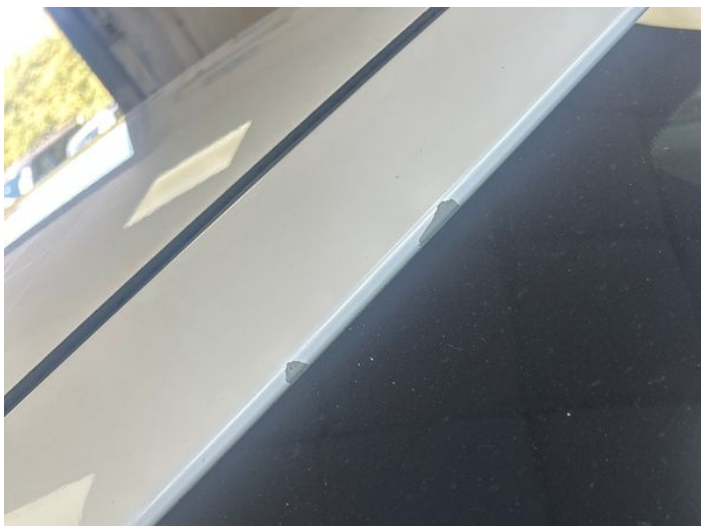
9: Roof Poor Previous Repair Paint Flake
