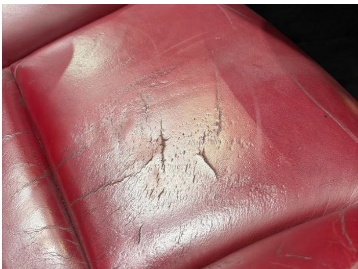
11: Seat Base Cover osf Torn Over 3mm
