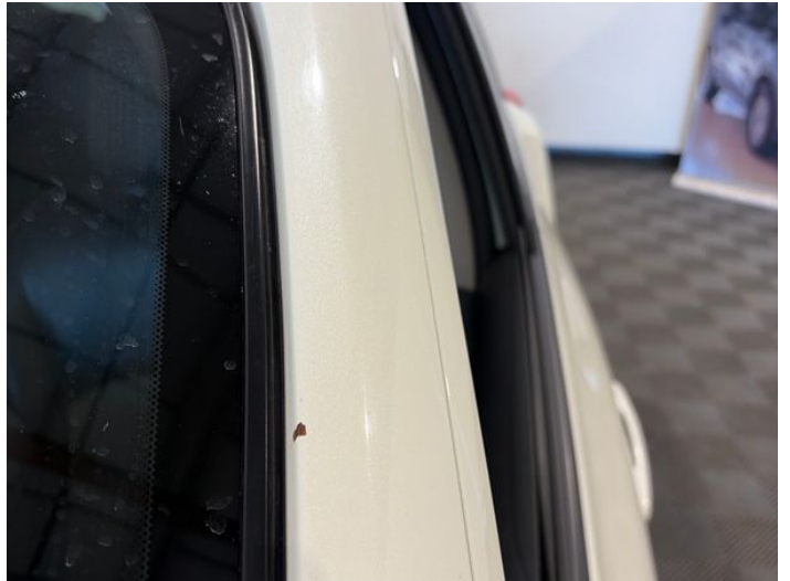
16: A Post ns Chipped Over 5mm
