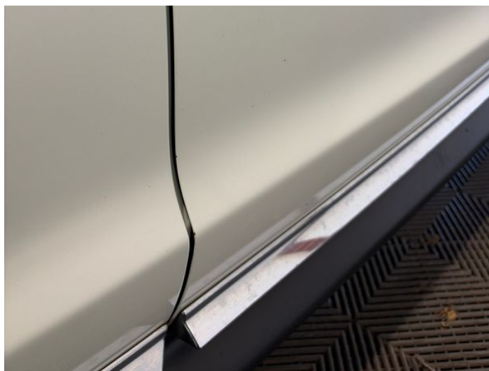
12: Door osf Chipped Edge Chip
