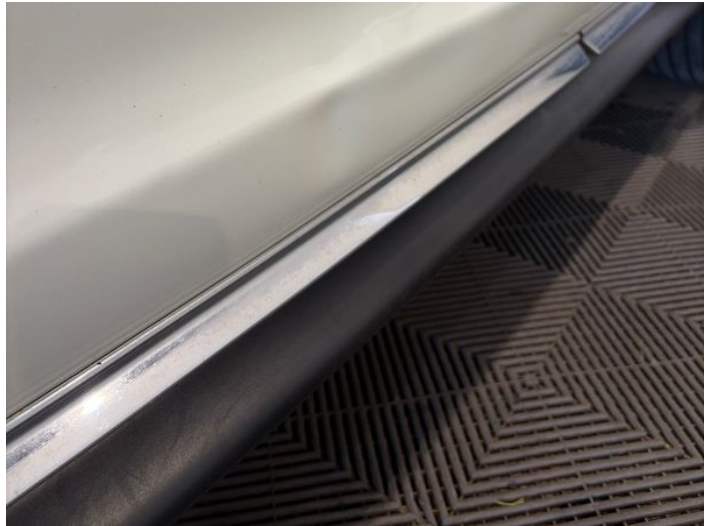
4: Door nsf Dented Over 30mm
