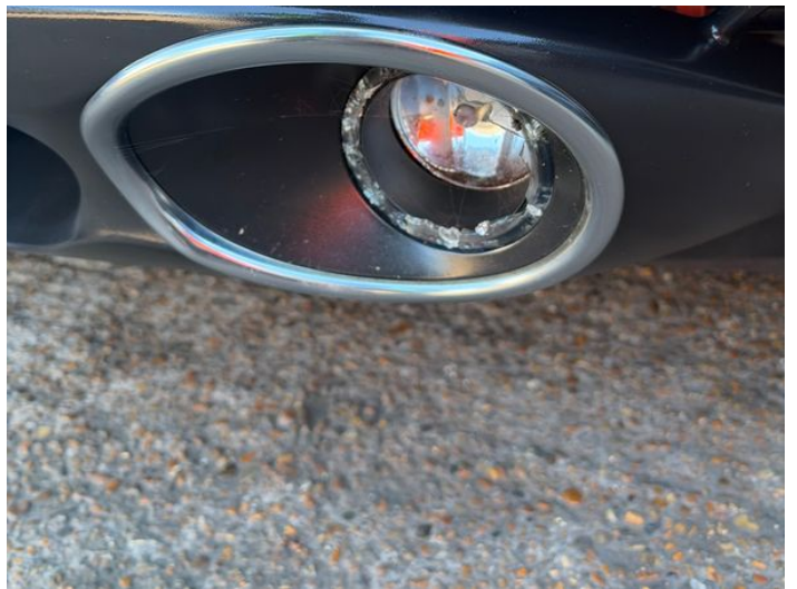
18: Fogdriving Lamp nsf Broken Replace
