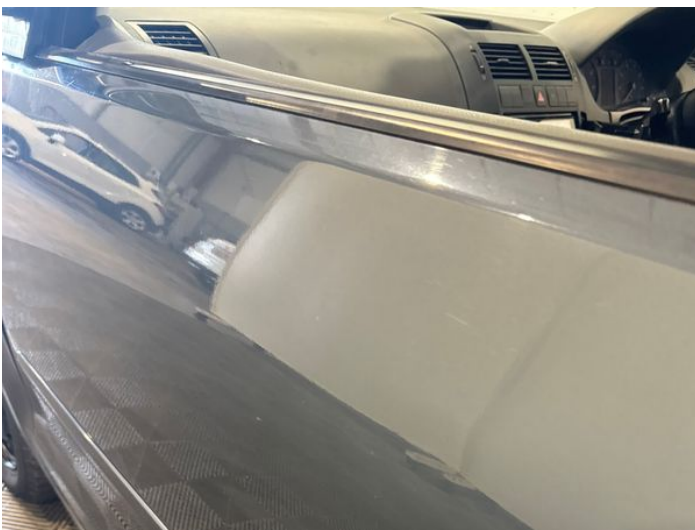
7: Door nsf Dented Over 30mm
