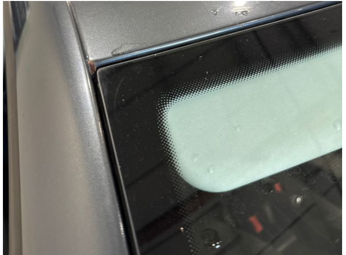
22: Roof Rusted Over 5mm
