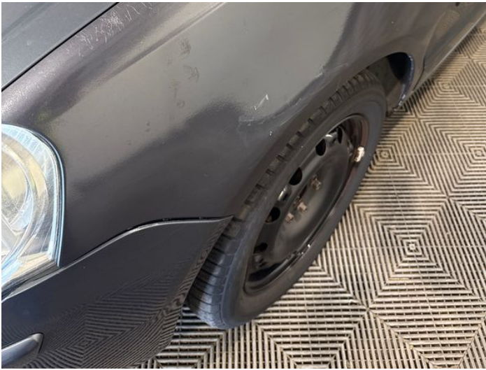
5: Wing nsf Poor Previous Repair Rippled UpTo 30%
