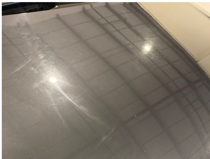
2: Bonnet Scratched Over 25mm Thru Paint
