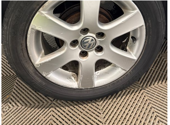
16: Wheel osr Scratched Over 50mm
