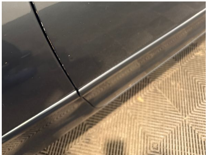
18: Door osf Dented Between 10mm + 30mm
