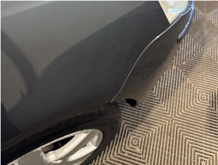
21: Wing osf Poor Previous Repair Poor Paint
