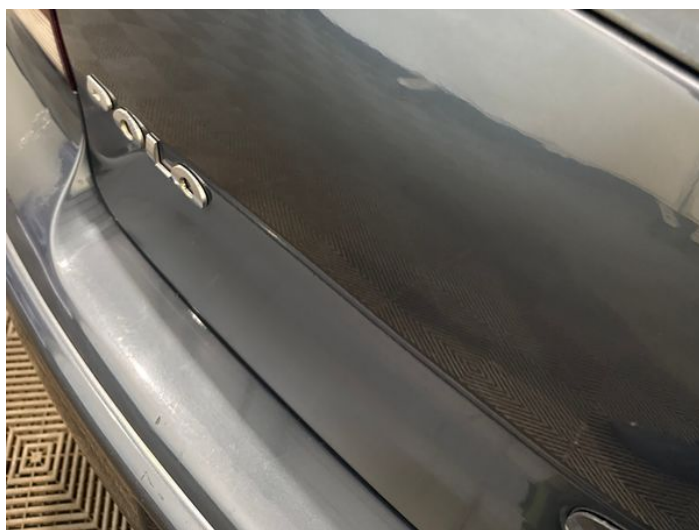
14: Tailgate Rusted Over 5mm
