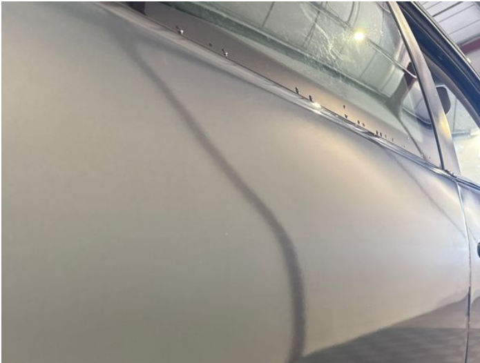
15: Qtr Panel osr Poor Previous Repair Rippled UpTo 30%
