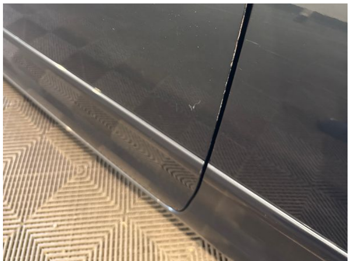
8: Door nsf Scratched Over 25mm Thru Paint
