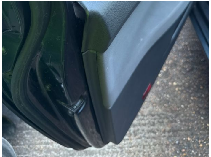
24: Door Pad nsf Scuffed Over 25mm
