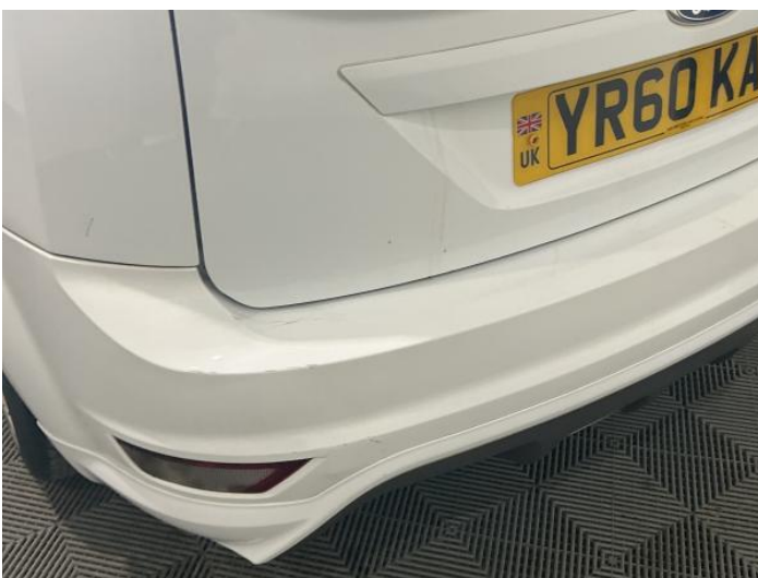
7: Bumper Rear Scratched Over 100mm Thru Paint
