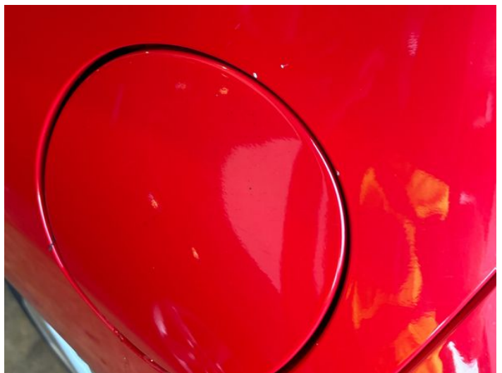
8: Qtr Panel nsr Chipped 1 To 5
