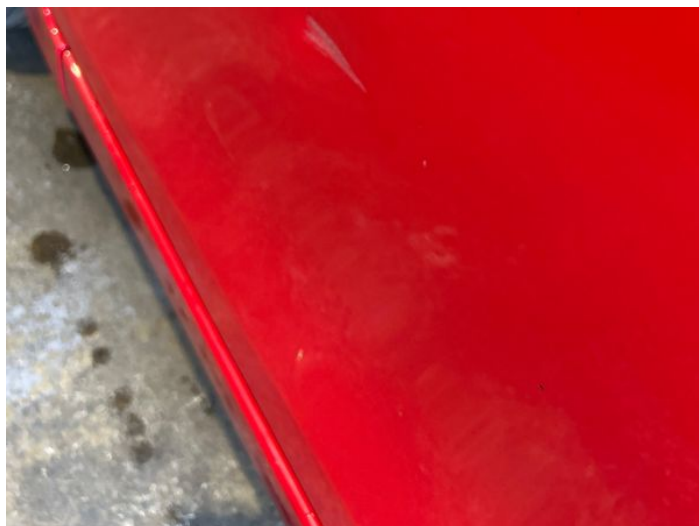
10: Door nsf Dented With Paint Damage
