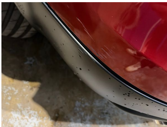
8: Bumper Rear Scratched 25 to 100mm Thru Paint
