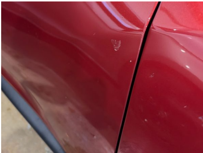
3: Door osf Poor Previous Repair Paint Flake
