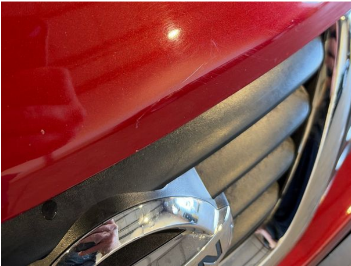
17: Bumper Front Scratched UpTo 25mm Thru Paint
