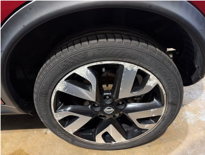
9: Wheel nsr Corroded Light
