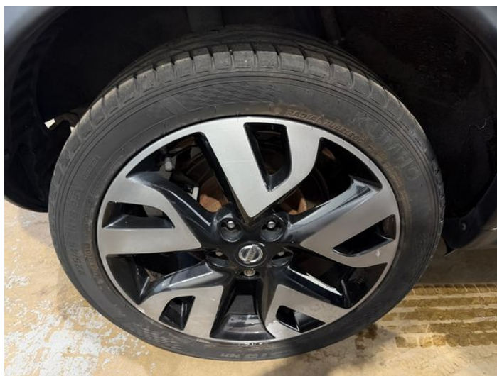
6: Wheel osr Corroded Light
