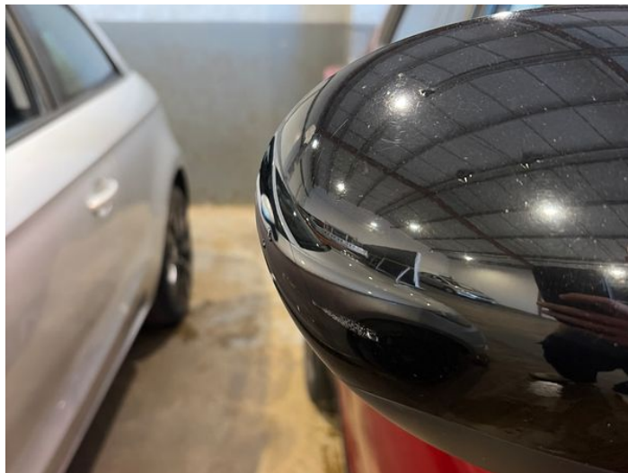
4: Door Mirror Assy osf Scratched (Painted) UpTo 25mm Thru Paint
