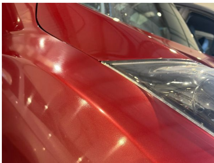
2: Wing osf Poor Previous Repair Poor Paint
