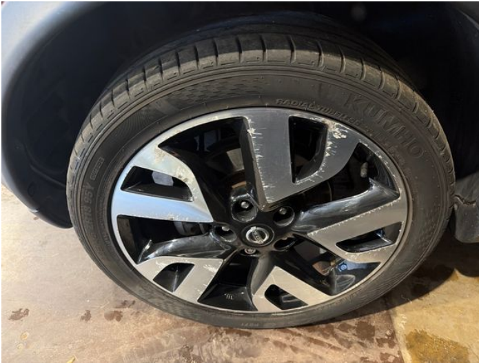
15: Wheel nsf Corroded Light
