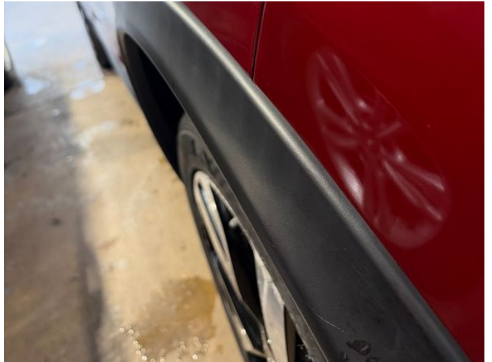
10: Qtr Panel nsr Dented 2 Or Less UpTo 10mm
