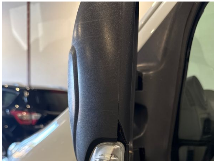
6: Door Mirror Assy nsf Broken Replace
