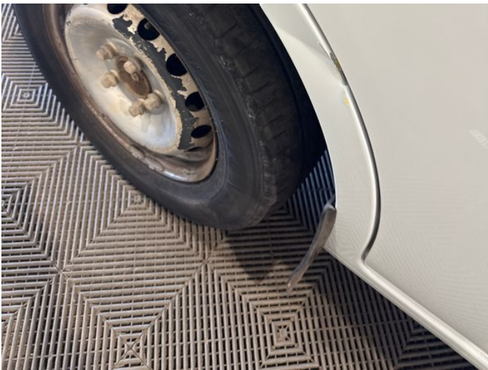
5: Sill ns Dented With Paint Damage
