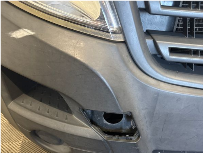
3: Front TowEye Cvr Missing Replace
