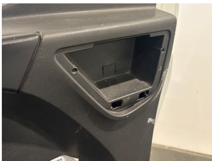
20: Fascia Trim Missing Replace
