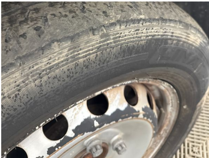
21: Tyre osf Damaged Replace
