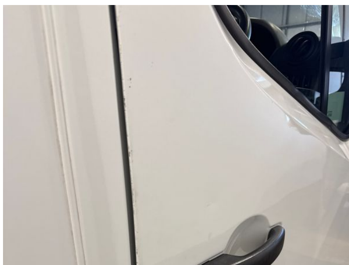
18: Door osf Dented With Paint Damage
