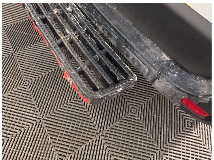
14: Bumper Rear Moulding Scuffed (Unpainted) Over 100mm
