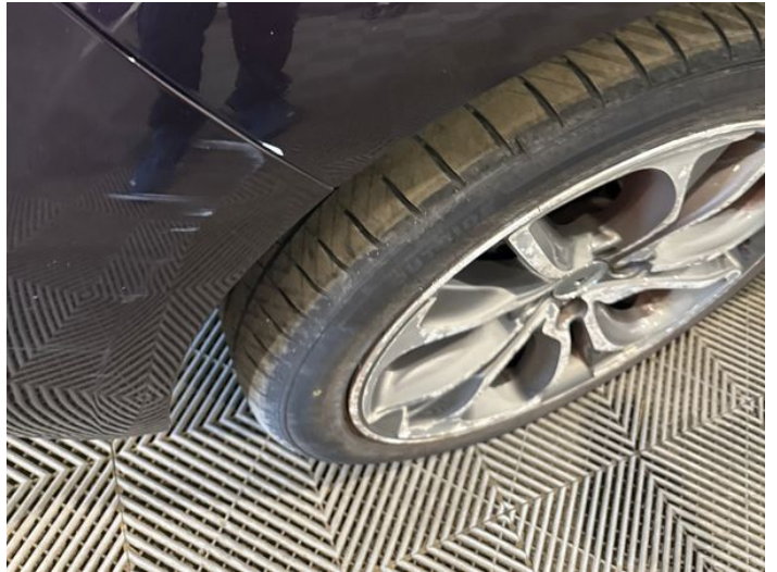
4: Wing nsf Scratched UpTo 25mm Thru Paint
