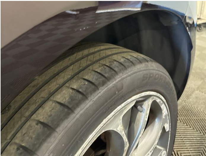
11: Qtr Panel nsr Dented Over 30mm
