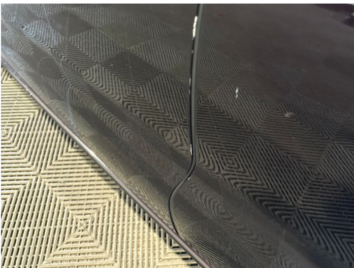
7: Door nsf Chipped Edge Chip
