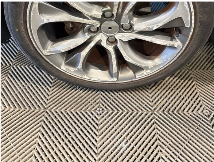
5: Wheel nsf Scratched Over 50mm
