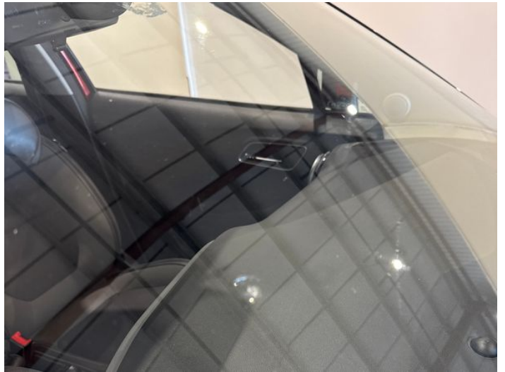
18: Screen Front Cracked Replace
