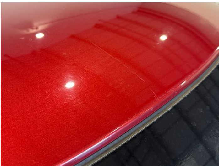
19: Roof Scratched Over 25mm Thru Paint
