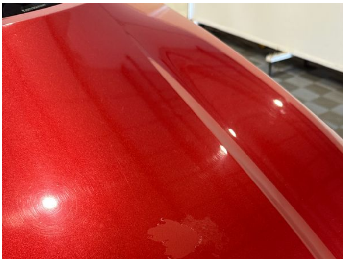
1: Bonnet Poor Previous Repair Paint Flake
