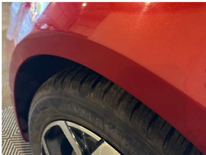
4: Wing nsf Poor Previous Repair Poor Paint
