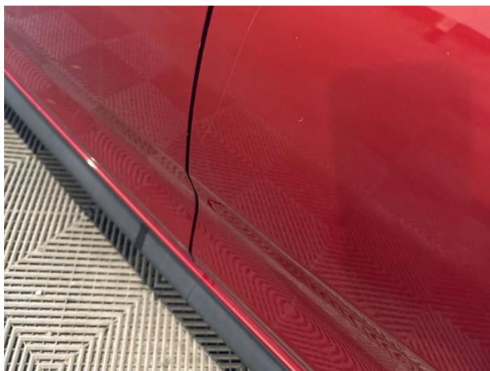
6: Door nsr Poor Previous Repair Rippled UpTo 30%
