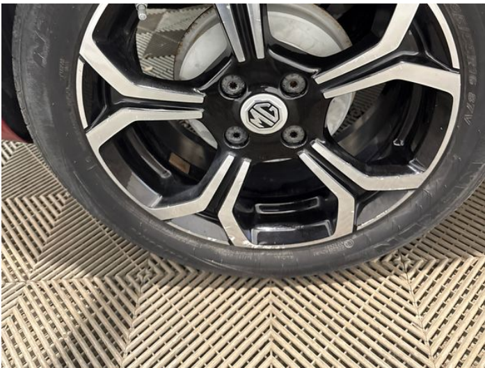
11: Wheel osr Scratched Over 50mm
