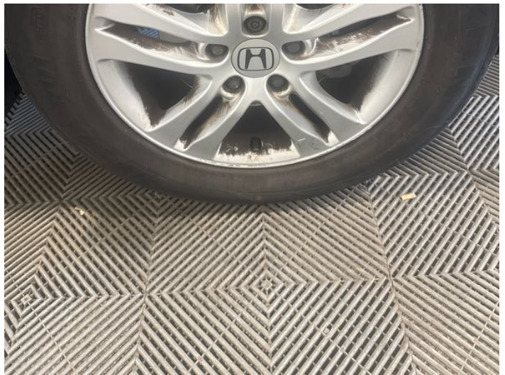
18: Wheel osf Scratched Over 50mm
