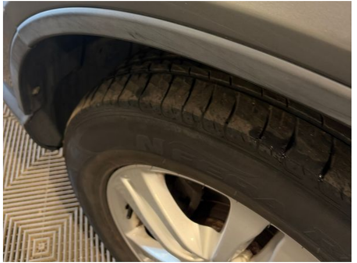
4: Wing nsf Scratched Over 25mm Thru Paint
