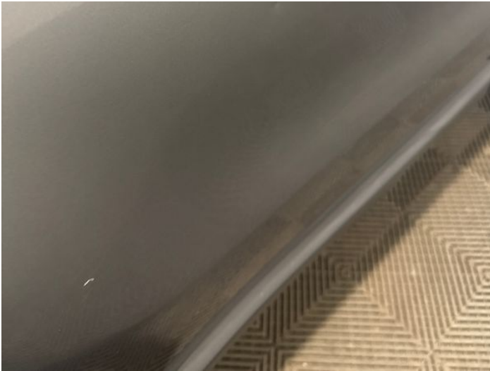
15: Door osr Dented Between 10mm + 30mm
