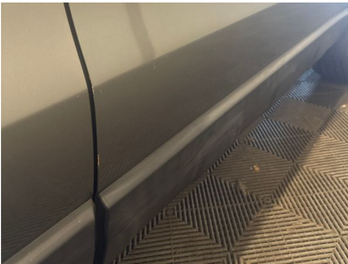
17: Door osf Scratched Over 25mm Thru Paint
