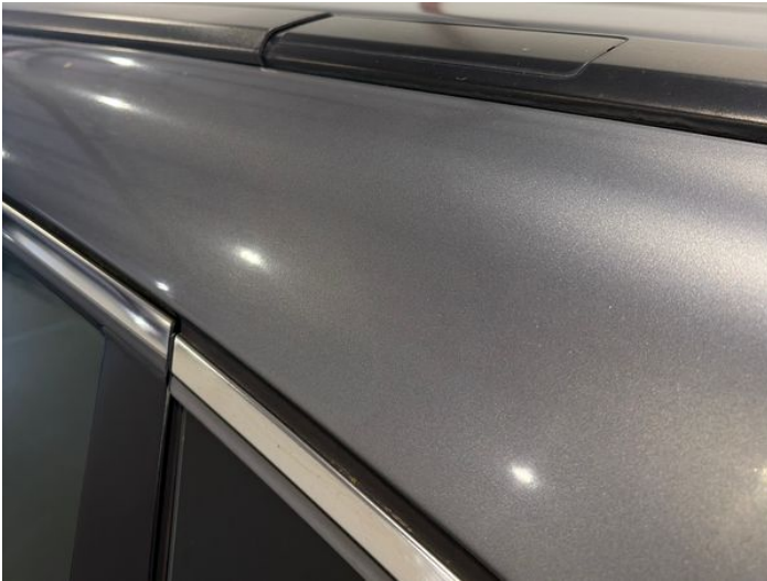
9: C Post ns Poor Previous Repair Poor Paint
