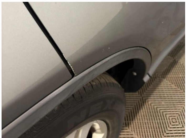
14: Door osr Chipped Edge Chip
