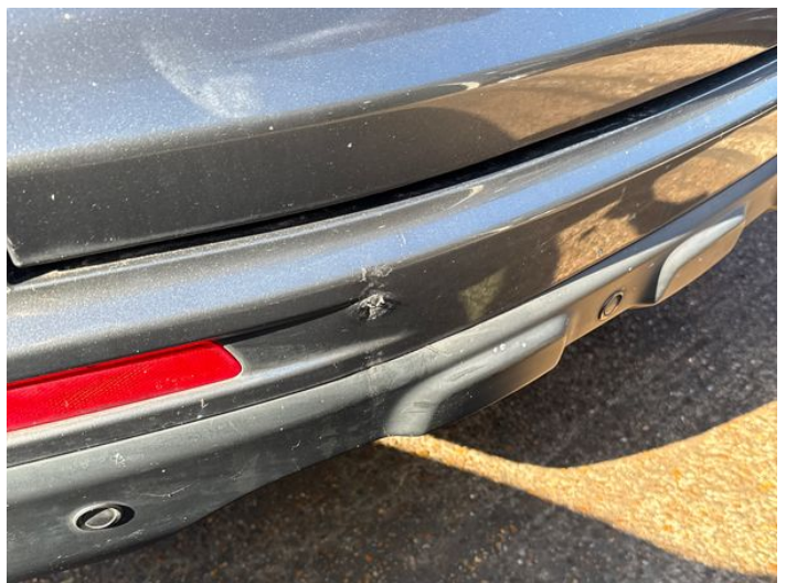
20: Bumper Rear Moulding Scuffed (Unpainted) Over 100mm
