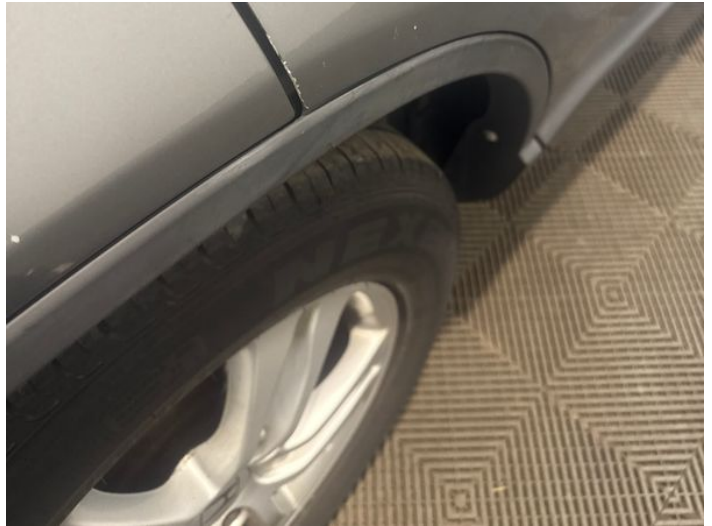
16: Door osr Chipped Edge Chip
