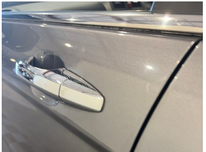
6: Door nsf Dented Between 10mm + 30mm
