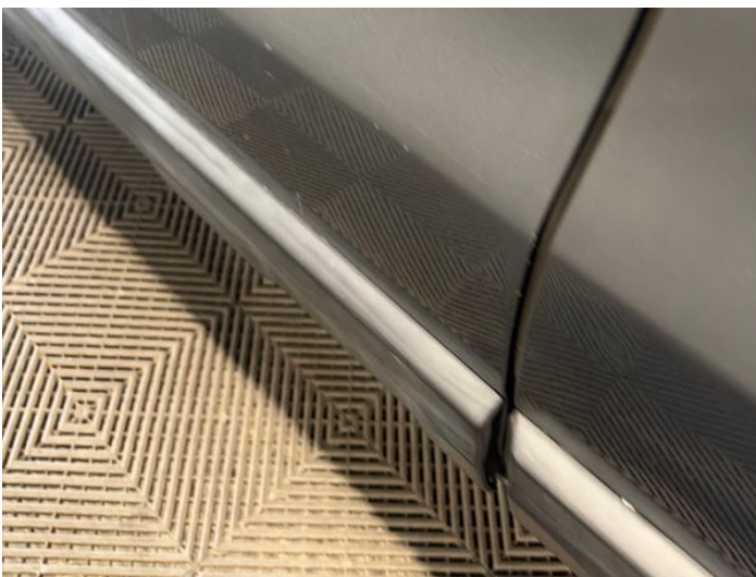
7: Door nsf Chipped 1 To 5
