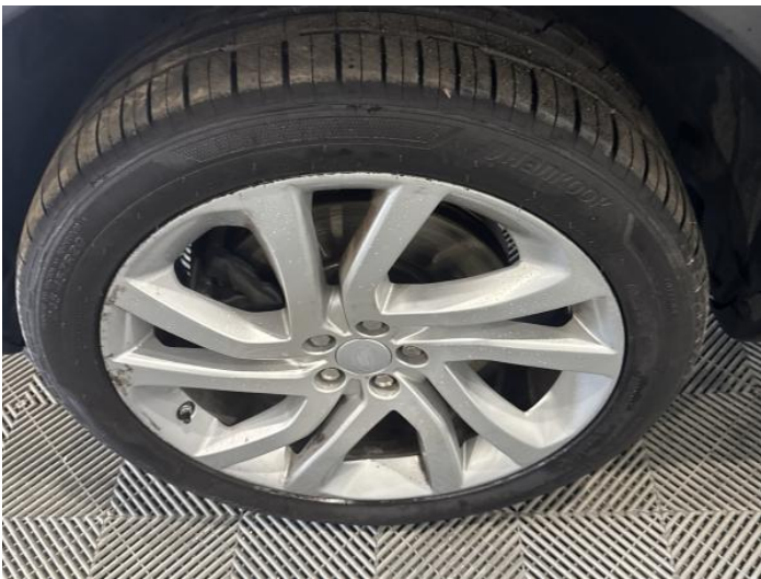
5: Wheel nsf Scratched Over 50mm
