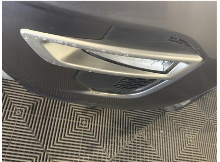
4: Bumper Front Moulding Scratched (Painted) Over 25mm Thru Paint
