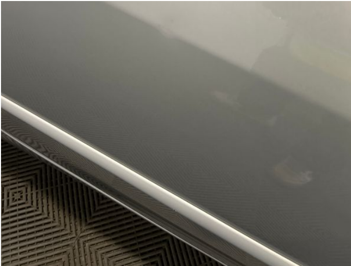
3: Door osr Dented Between 10mm + 30mm
