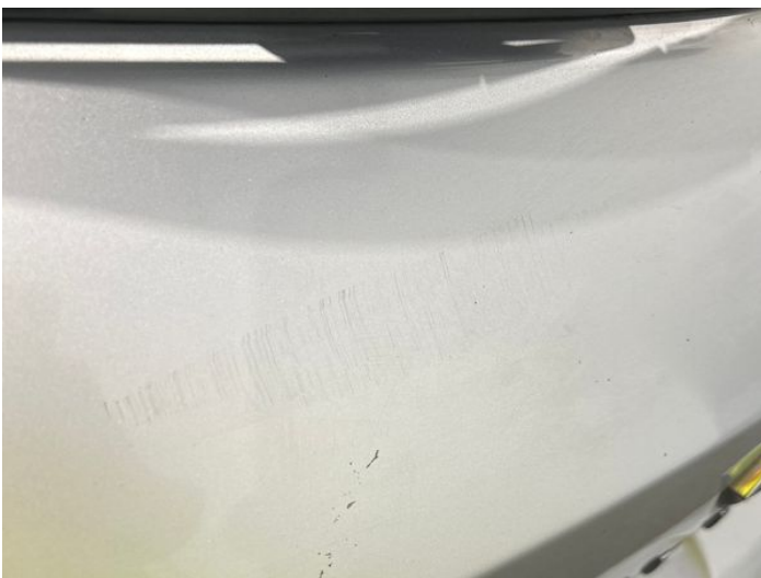
7: Tailgate Scratched Over 25mm Thru Paint
