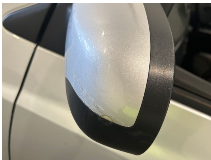
14: Door Mirror Assy nsf Scratched (Painted) Over 25mm Thru Paint
