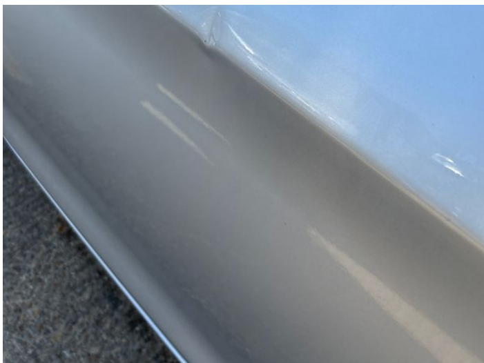
3: Door osf Dented Over 30mm
