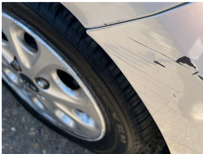
2: Wing osf Scratched UpTo 25mm Thru Paint
