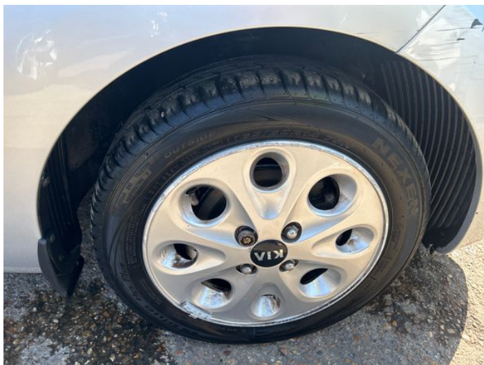
1: Wheel osf Scratched Over 50mm
