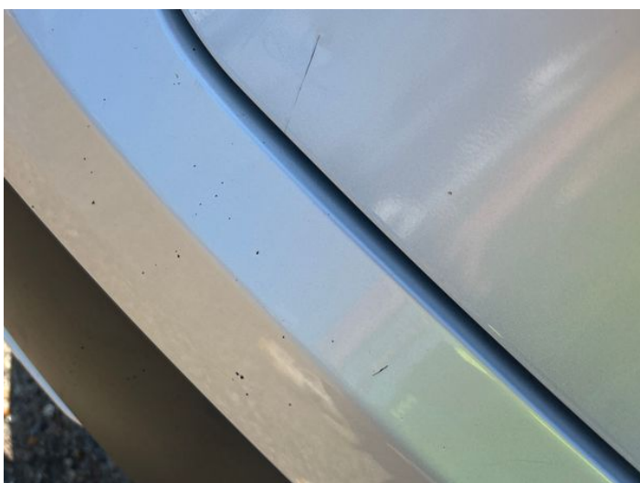
5: Tailgate Scratched Over 25mm Thru Paint
