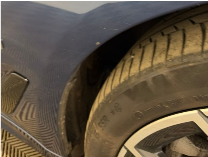
11: Wing osf Scratched UpTo 25mm Thru Paint
