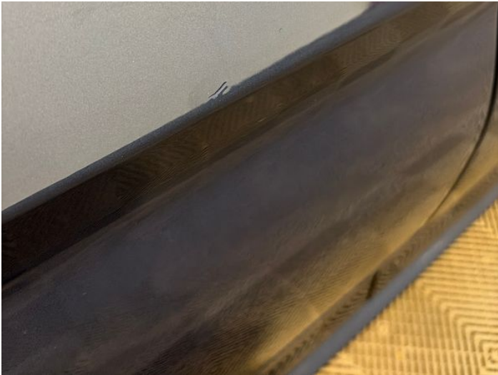
9: Door osr Scratched UpTo 25mm Thru Paint
