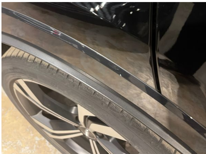
3: Qtr Panel osr Chipped 1 To 5
