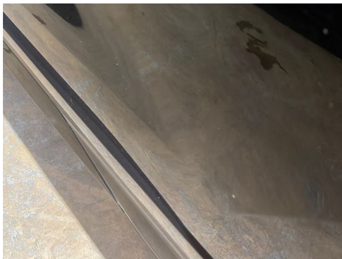
4: Door nsr Dented Over 30mm
