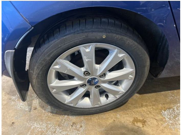
6: Wheel osr Scratched Over 50mm
