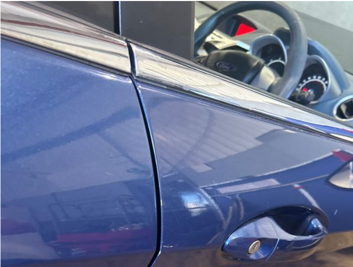
3: Door osf Chipped Edge Chip
