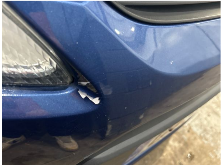
16: Bumper Front Poor Previous Repair Paint Flake
