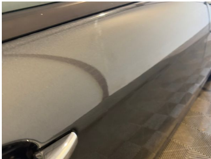
10: Door osr Dented Between 10mm + 30mm
