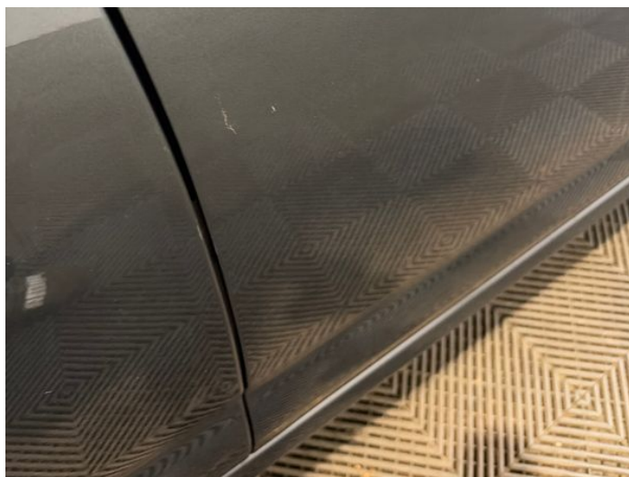
12: Door osf Scratched UpTo 25mm Thru Paint
