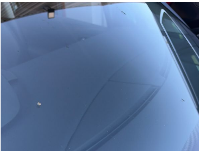
19: Screen Front Chipped Over 10mm
