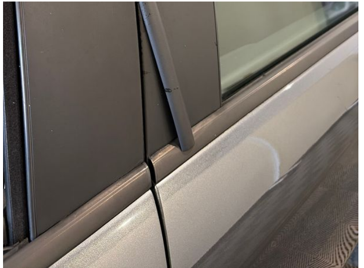
18: Aperture Seal nsr Broken Replace
