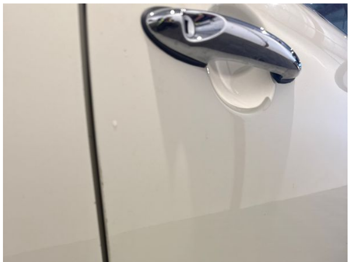
14: Door osf Chipped Edge Chip
