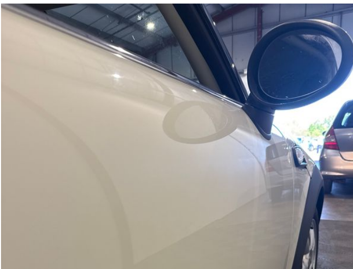
13: Door osf Dented Between 10mm + 30mm
