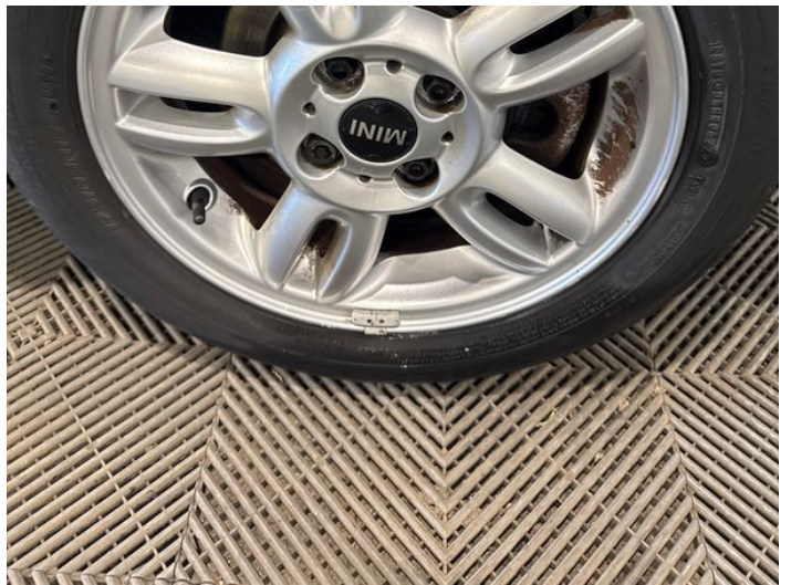
6: Wheel nsr Scratched Up To 50mm
