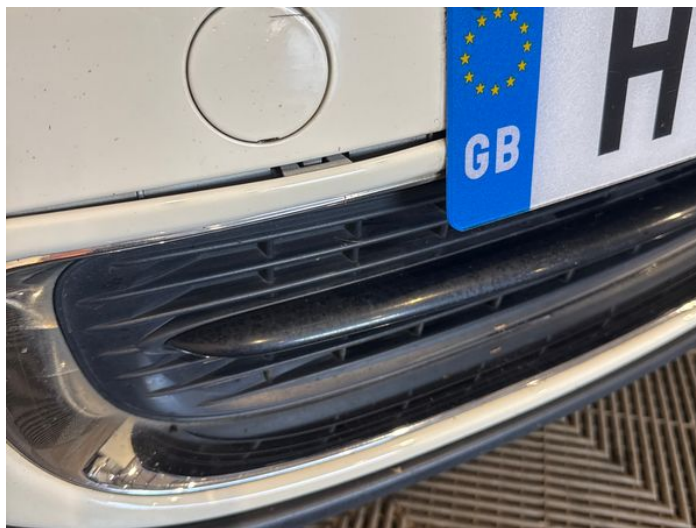
2: Bumper Front Moulding Broken Replace
