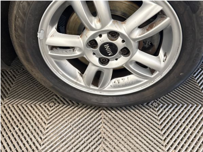
15: Wheel osf Scratched Over 50mm
