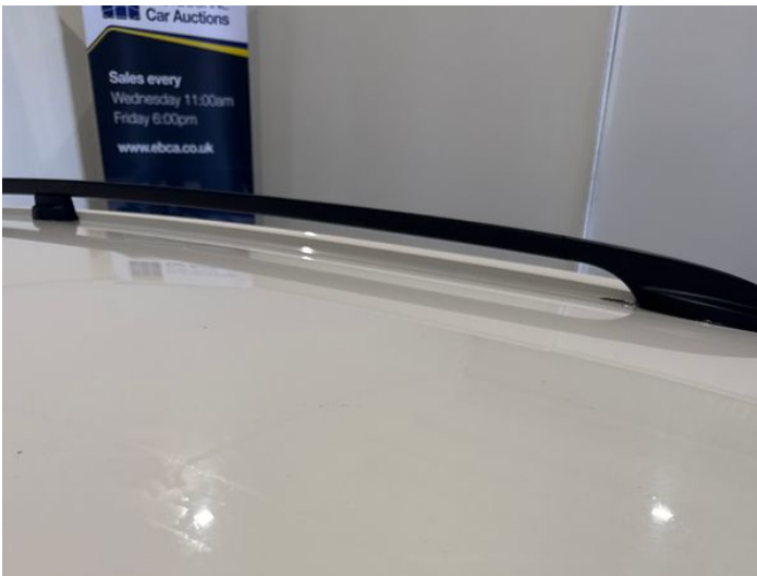
11: Roof Dented Between 10mm + 30mm
