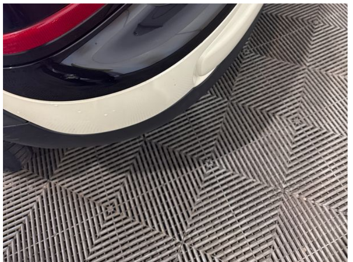
8: Bumper Rear Scratched 25 to 100mm Thru Paint
