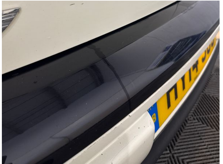
10: Tailgate Scratched UpTo 25mm Thru Paint
