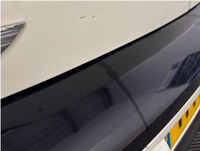
9: Tailgate Dented 2 Or Less UpTo 10mm
