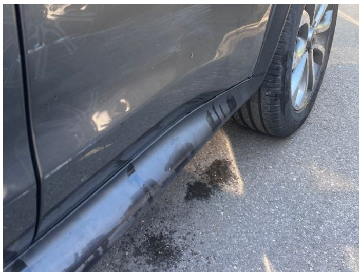
6: Door nsr Dented Between 10mm + 30mm
