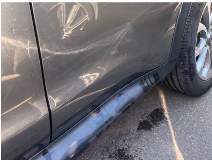
5: Door nsr Scratched Over 25mm Thru Paint
