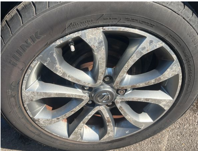
11: Wheel osr Corroded Light
