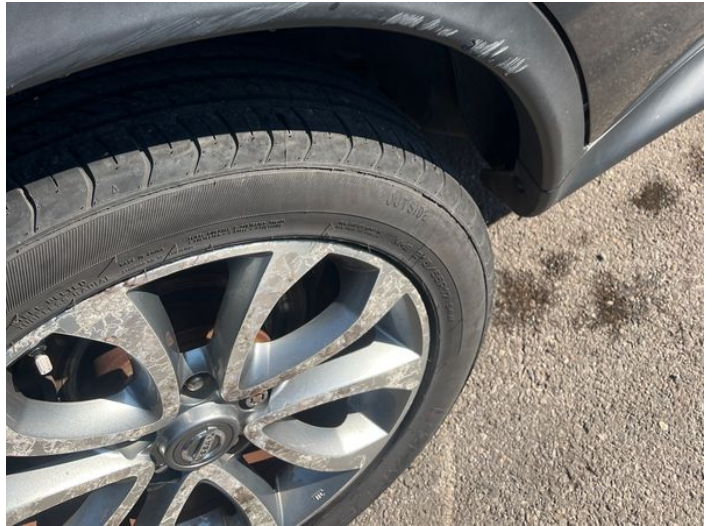
10: Wheel Trim osr Scratched Over 50mm
