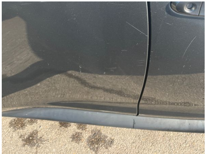
12: Door osr Scratched Over 25mm Thru Paint
