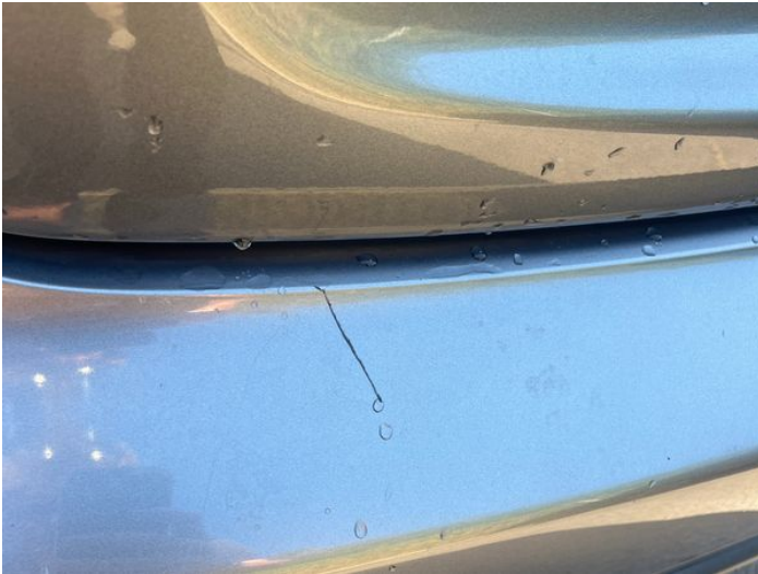
9: Bumper Rear Scratched Over 100mm Thru Paint
