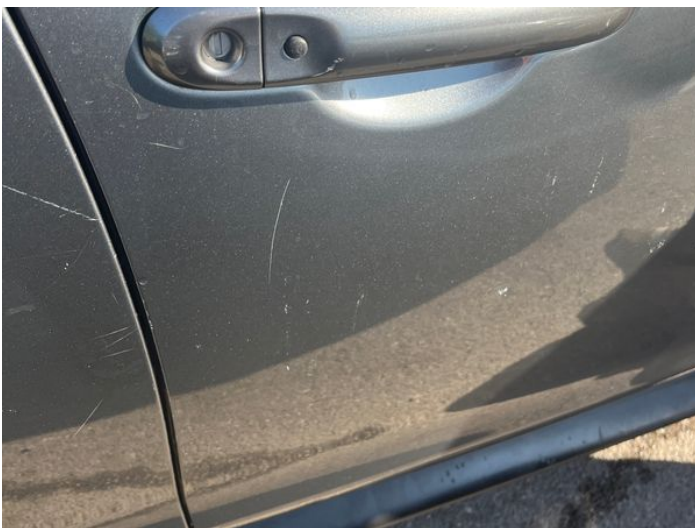
13: Door osf Scratched Over 25mm Thru Paint
