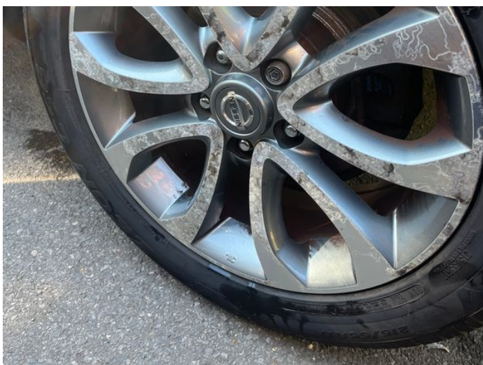
7: Wheel nsr Corroded Light
