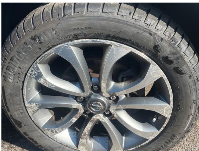
1: Wheel of front left Scratched Over 50mm
