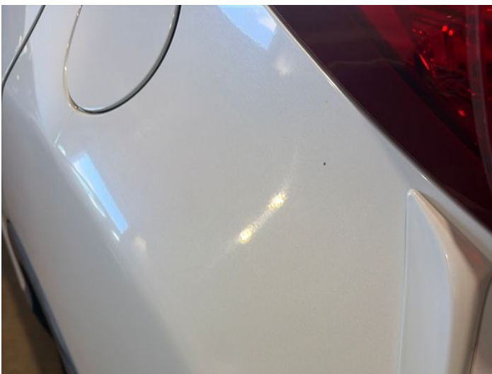
7: Qtr Panel nsr Dented Between 10mm + 30mm
