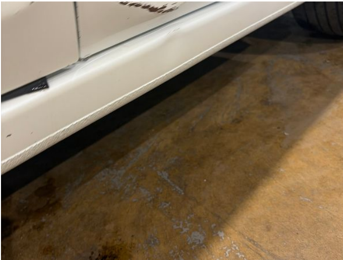
5: Sill ns Dented Over 30mm
