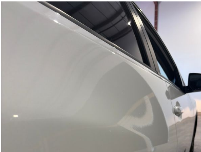
11: Door osr Dented With Paint Damage
