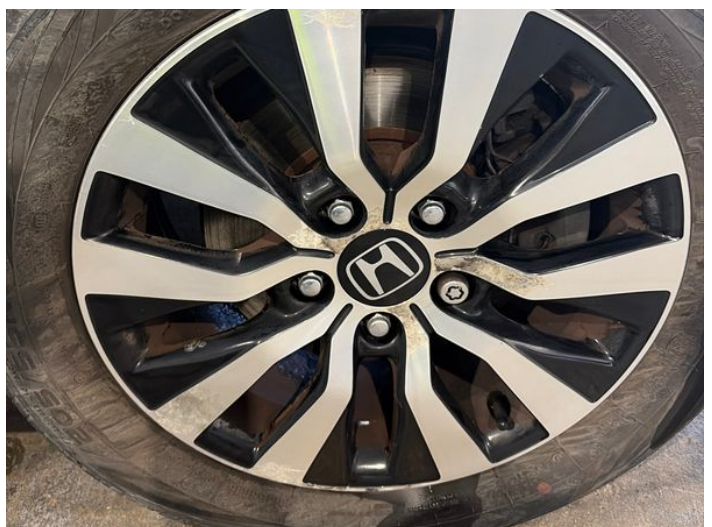
14: Wheel osf Scratched Over 50mm
