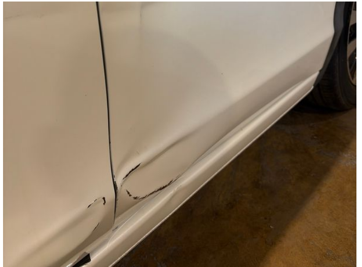
6: Door nsr Dented With Paint Damage
