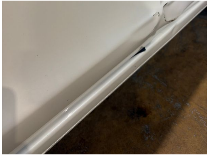
4: Door nsf Dented With Paint Damage
