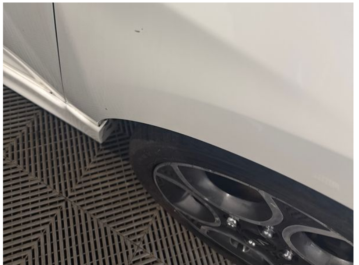
18: Wing osf Scratched UpTo 25mm Thru Paint
