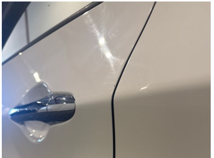
6: Door nsf Chipped Edge Chip
