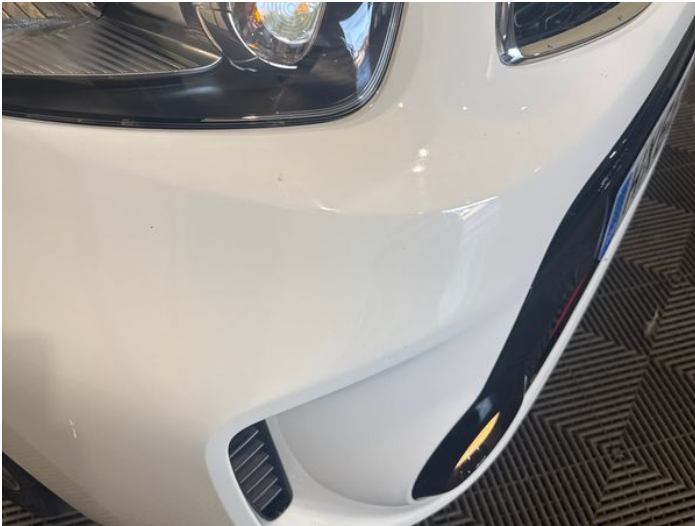
3: Bumper Front Poor Previous Repair Poor Paint
