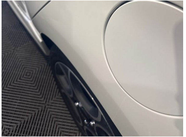
10: Qtr Panel nsr Dented Between 10mm + 30mm
