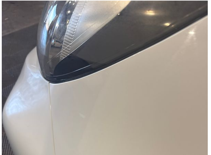
4: Wing nsf Scratched UpTo 25mm Thru Paint
