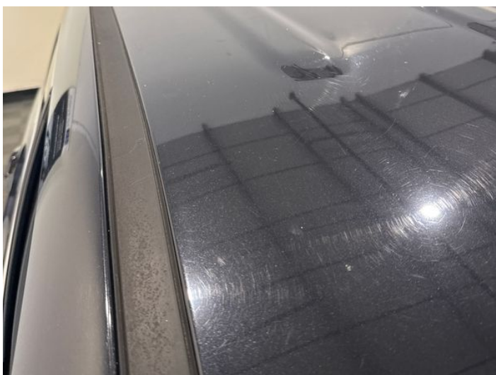
19: Roof Dented Between 10mm + 30mm
