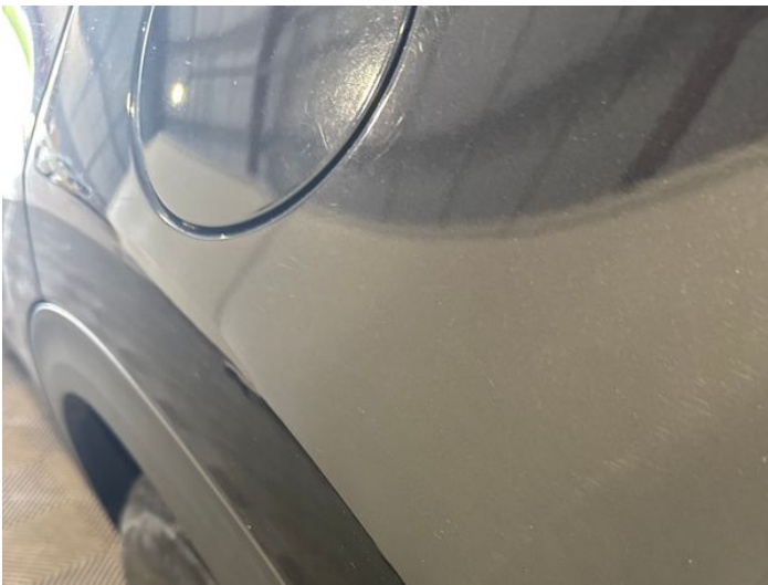
11: Qtr Panel nsr Dented Between 10mm + 30mm
