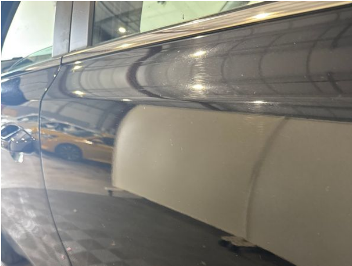
9: Door nsr Dented Over 30mm
