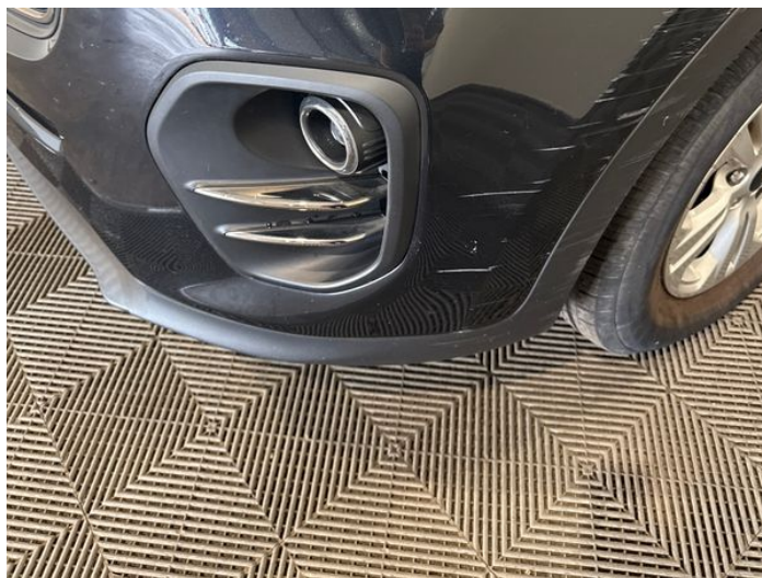
2: Bumper Front Scratched Over 100mm Thru Paint
