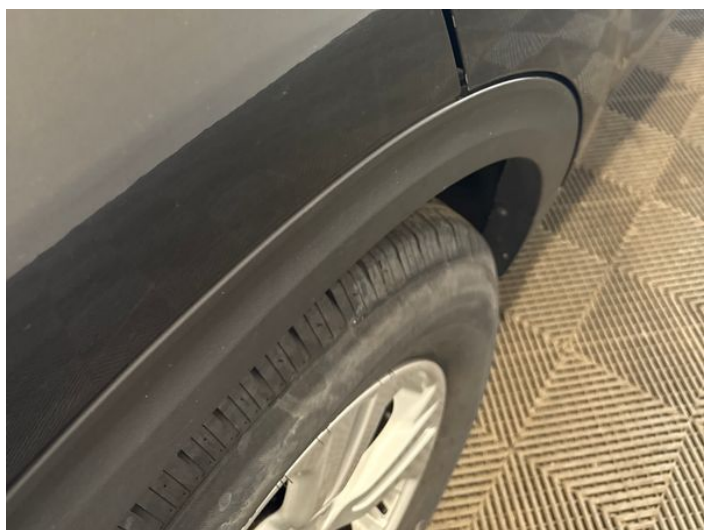
14: Qtr Panel osr Dented Between 10mm + 30mm
