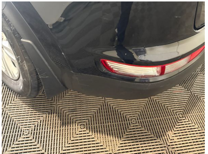
12: Bumper Rear Scratched Over 100mm Thru Paint
