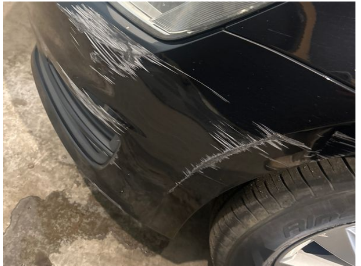
12: Bumper Front Scratched Over 100mm Thru Paint
