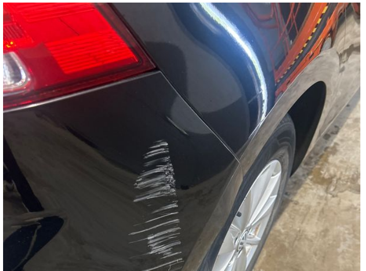
6: Bumper Rear Scratched Over 100mm Thru Paint
