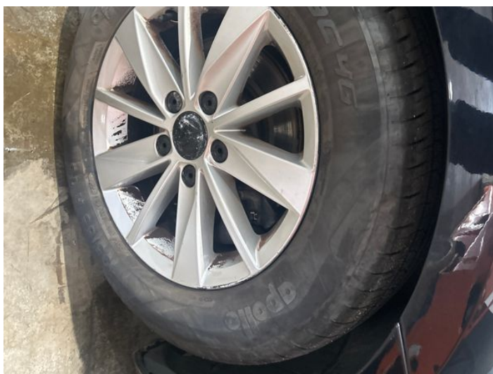
1: Wheel osf Scratched Over 50mm
