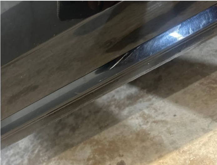
3: Sill os Scratched Over 25mm Thru Paint
