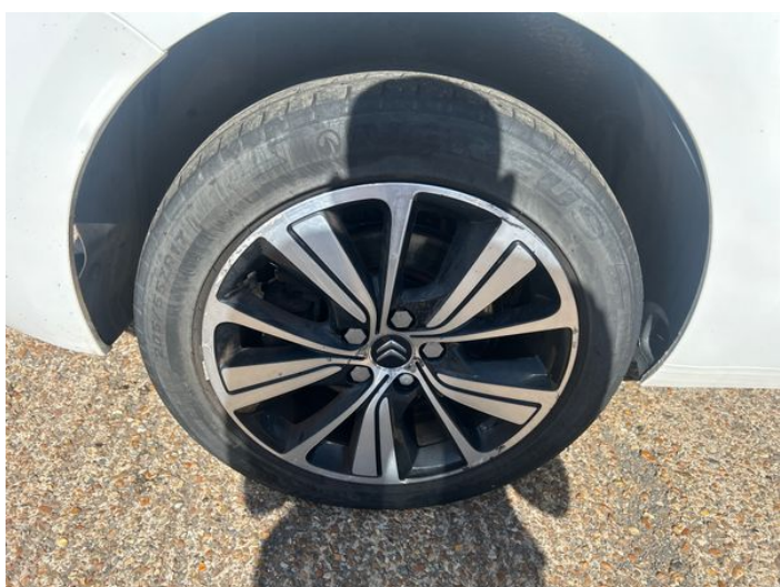
7: Wheel osr Corroded Light
