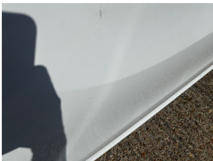
6: Door osr Scratched UpTo 25mm Thru Paint
