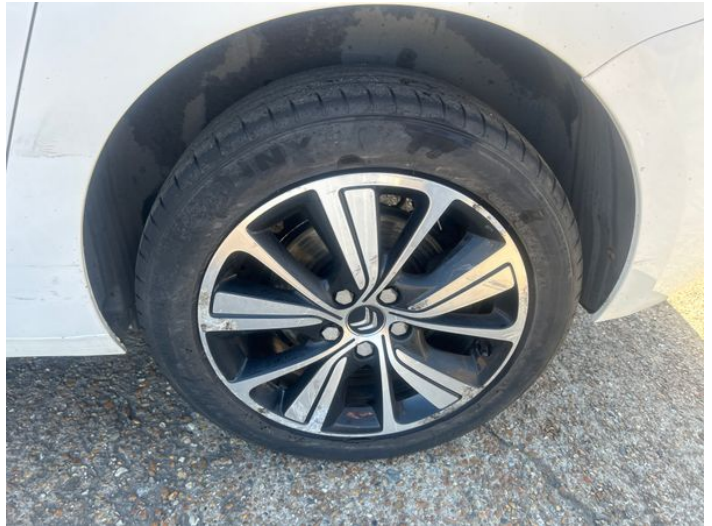
10: Wheel nsr Corroded Light
