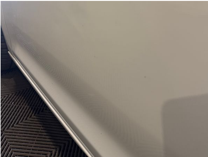
5: Door nsf Dented Over 30mm
