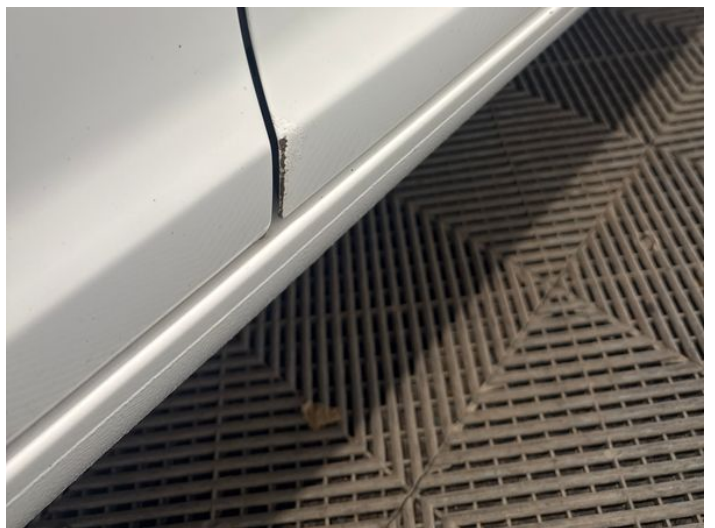
14: Door osf Scratched Rusted
