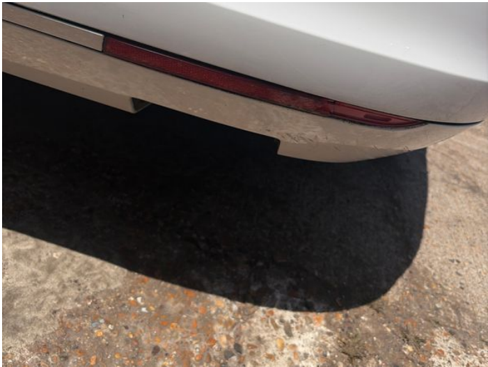
18: Rear TowEye Cvr Missing Replace
