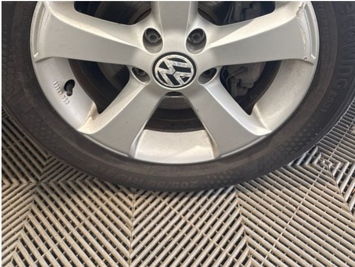
16: Wheel osf Scratched Over 50mm
