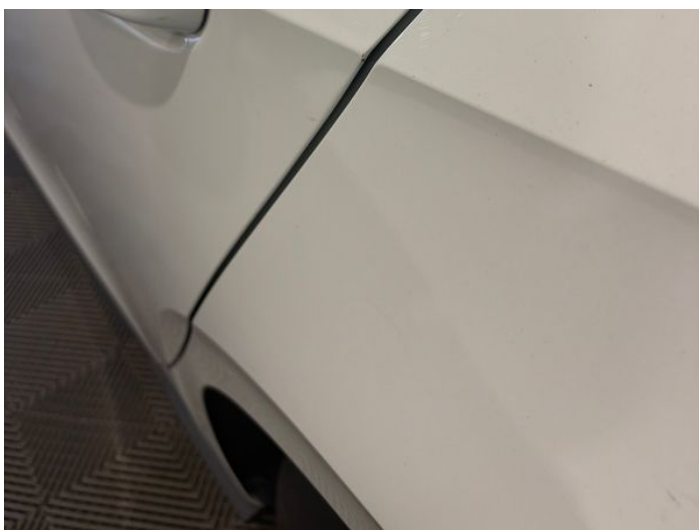
7: Door nsr Chipped Edge Chip
