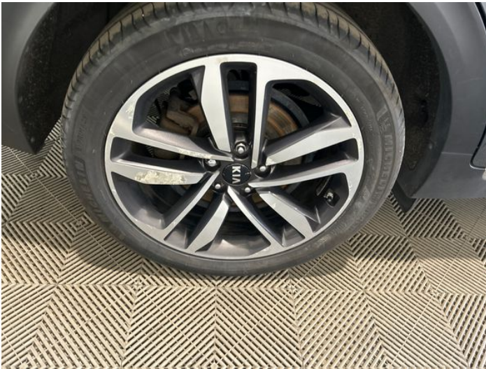
5: Wheel osr Corroded Light
