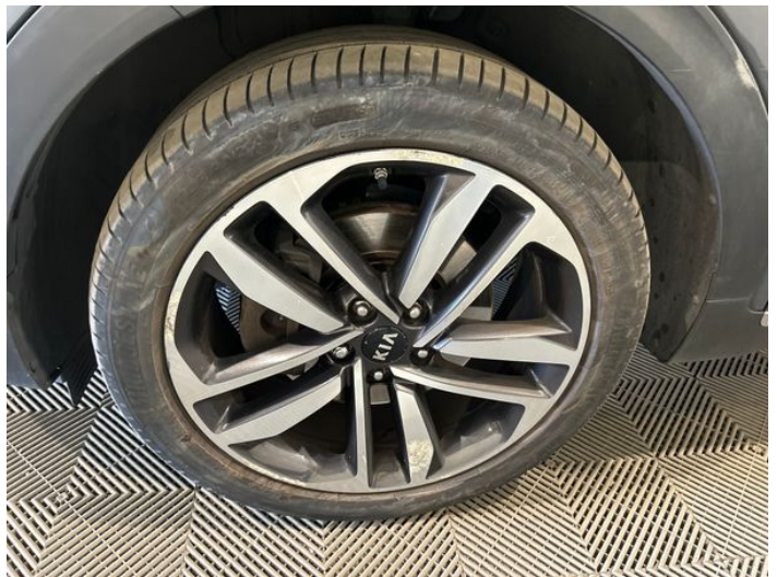
10: Wheel nsf Corroded Light
