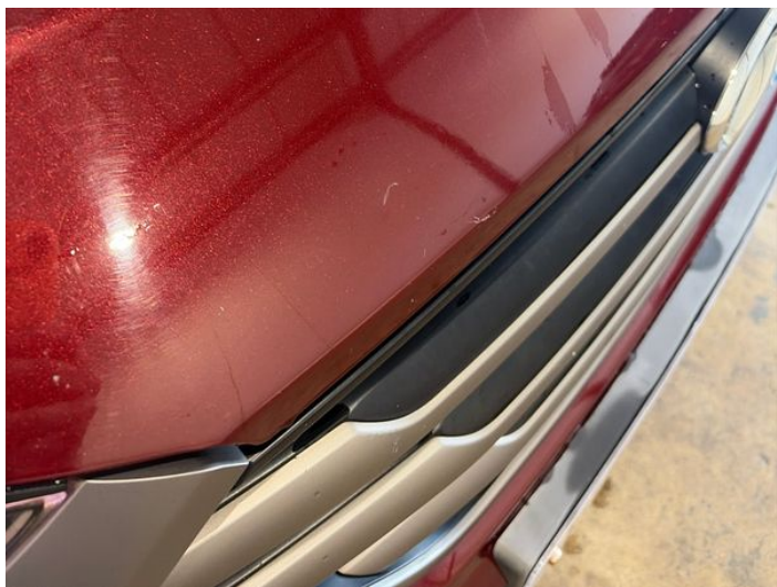
1: Bonnet Dented Between 10mm + 30mm
