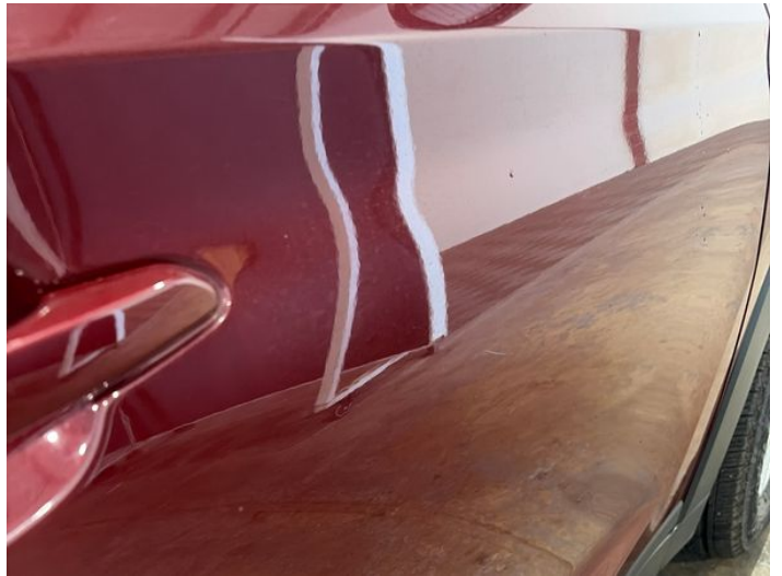
18: Door osf Scratched Over 25mm Thru Paint
