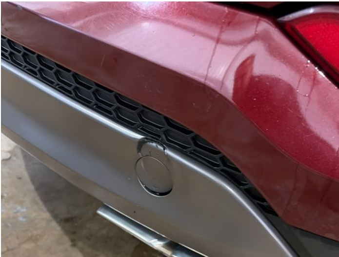
11: Bumper Rear Moulding Broken Replace
