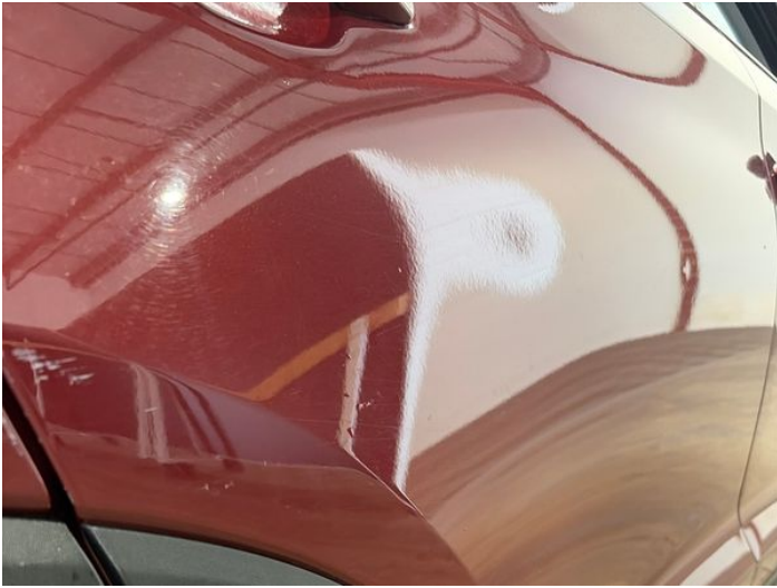
15: Door osr Scratched Over 25mm Thru Paint
