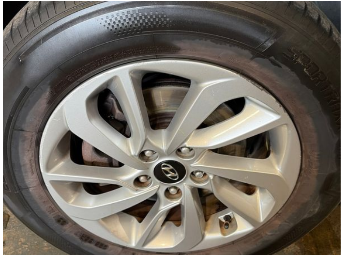
4: Wheel nsf Scratched Over 50mm
