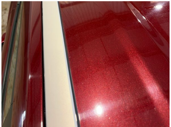
22: Roof Dented Over 30mm
