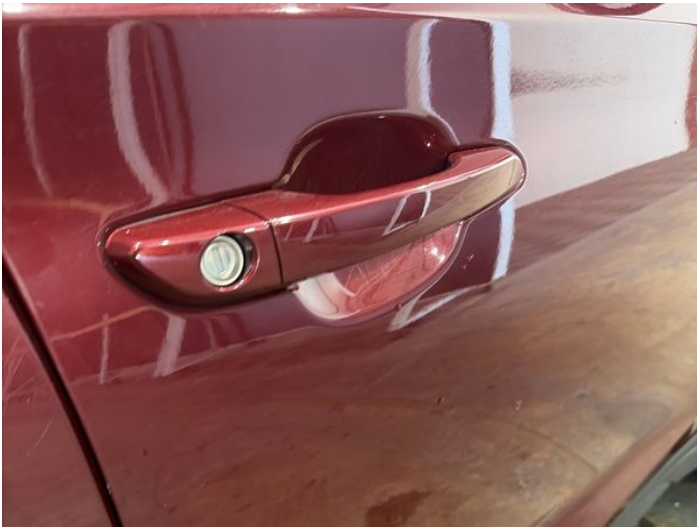
17: Door osf Dented Between 10mm + 30mm
