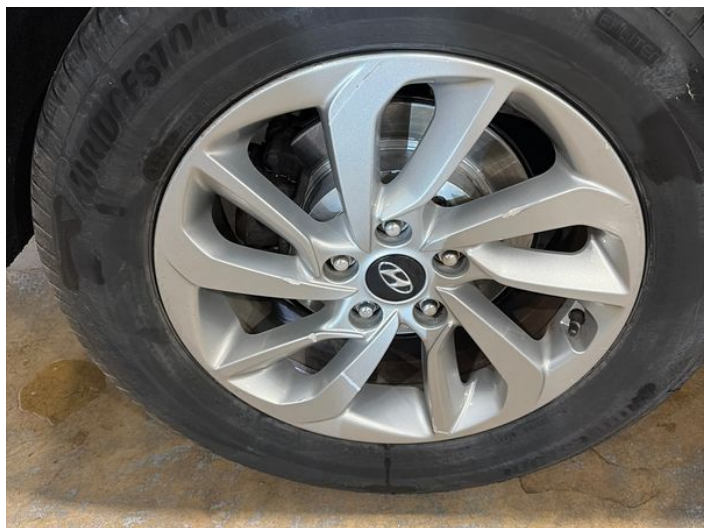
14: Wheel osr Scratched Over 50mm
