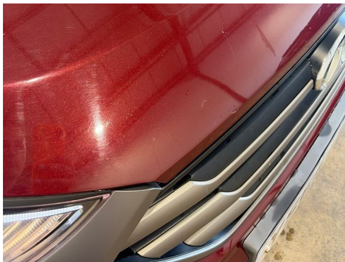
2: Bonnet Chipped Multiple Chips
