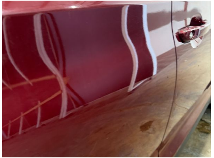
16: Door osr Dented Between 10mm + 30mm
